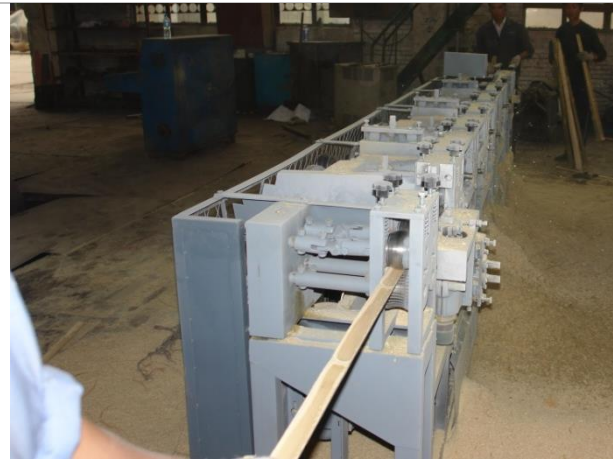
Fig. 2. Arc shape and milling machine
