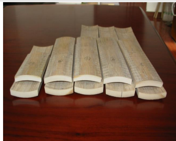
Fig. 3. Bamboo sheets without the outer part and inner part of bamboo
