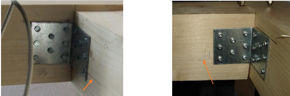
Fig. 17. Types of failures for variants A and C (Note: Orange arrows show visible cracks on loaded elements)
