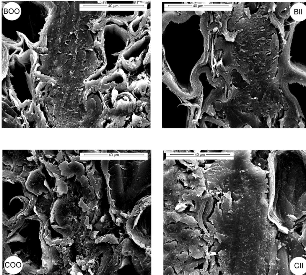
**Fig. 3.** Morphology of the bonding interface between parenchyma cells of the four kinds of bamboo laminated lumber
