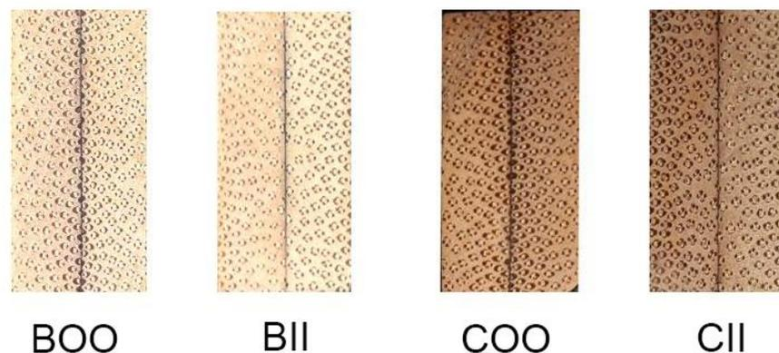
**Fig. 1.** Assembly patterns: (BOO) bleached bamboo, outer-to-outer; (BII) bleached bamboo, inner-to-inner; (COO) carbonized bamboo, outer-to-outer; (CII) carbonized bamboo, inner-to-inner
