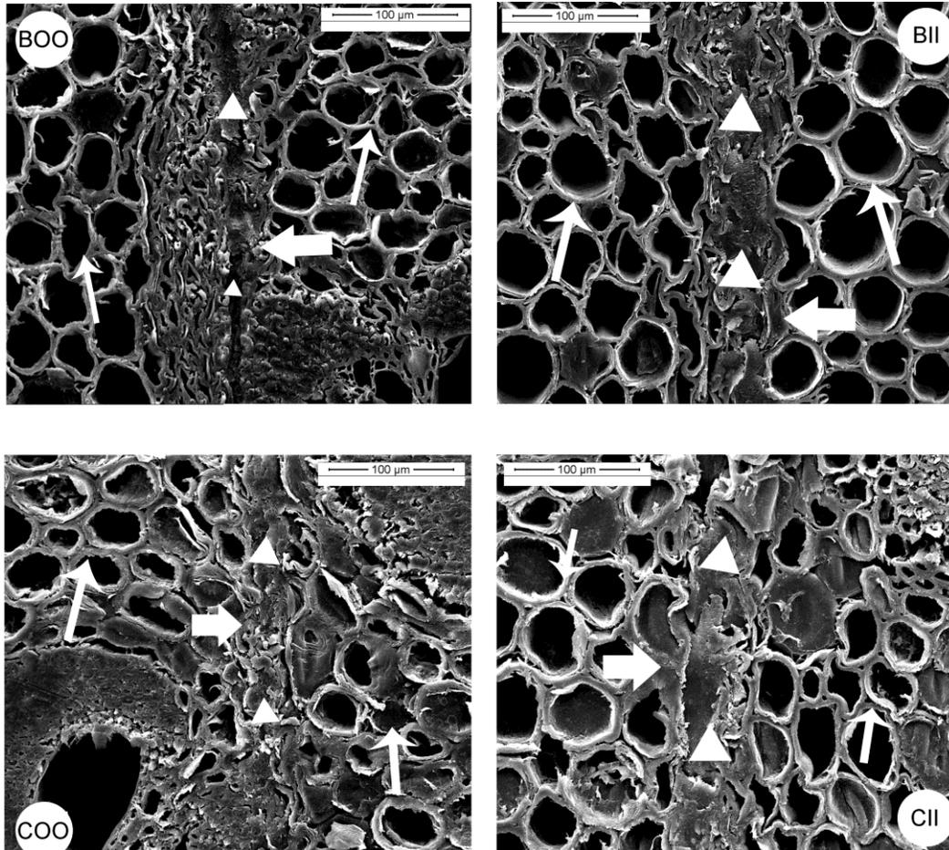
**Fig. 2.** SEM images of the bonding interface of the four kinds of bamboo laminated lumber. The triangles, coarse arrows, and thin arrows indicate the pure PF bond-line, the adhesive between cell walls, and the parenchyma cells without adhesive, respectively.
