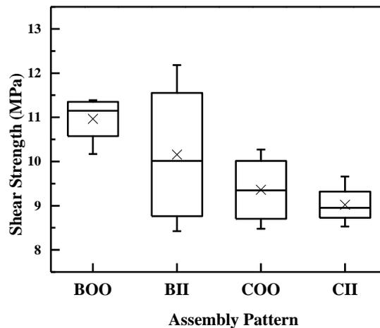
Fig. 6. Shear strength of the four kinds of bamboo laminated lumber
