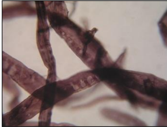
Fig. 2. Sulphite pulp (F2) stained by Herzberg stain
