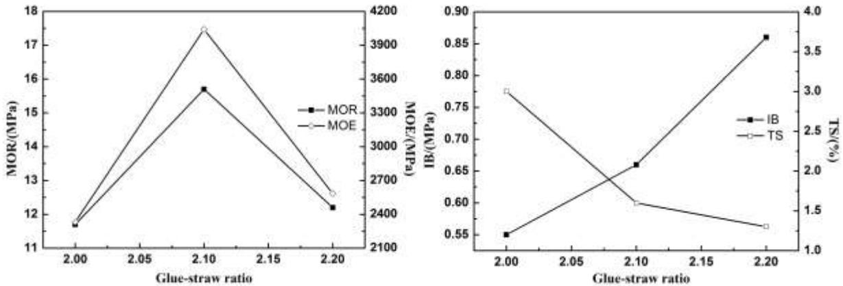
Fig. 1. Physical and mechanical properties of inorganic wheat-straw composite board
