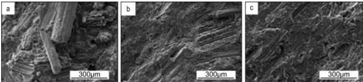
Fig. 2. SEM images of inorganic wheat-straw composite board fracture surface
