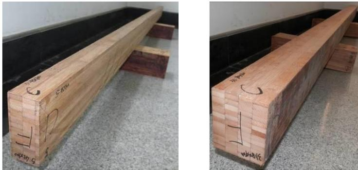
**Fig. 1.** Structural laminated bamboo
