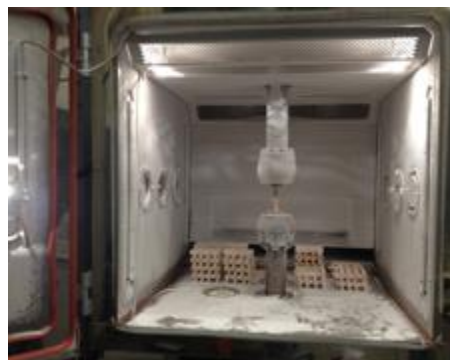
Fig. 2. Climate chamber, shear test machine, and test specimens
