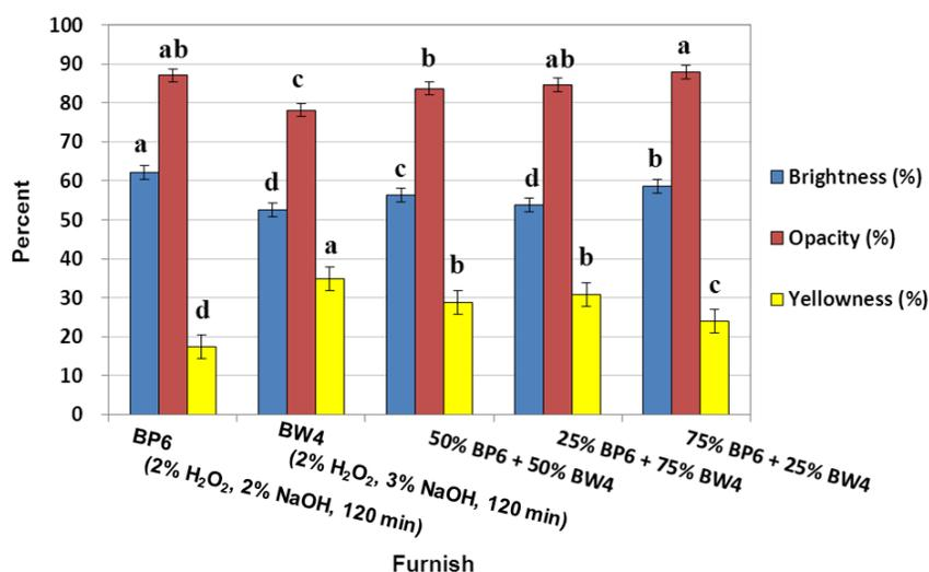
Fig. 2. Optical properties of pure and blended BSWP and BWPP
