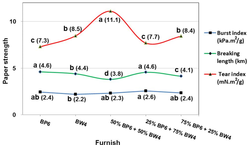
Fig. 3. Comparison of strength handsheets made from various ratios of BSWP and BWPP
