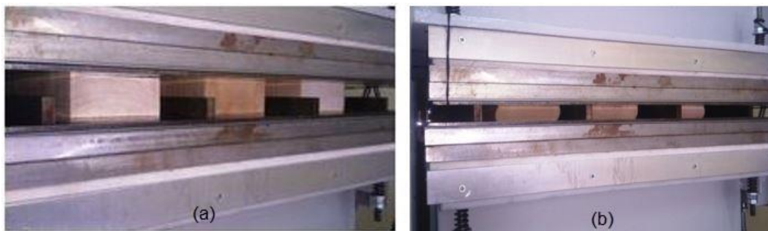
Fig. 1. (a) Heating of the samples before compression; (b) compression of the heated samples
