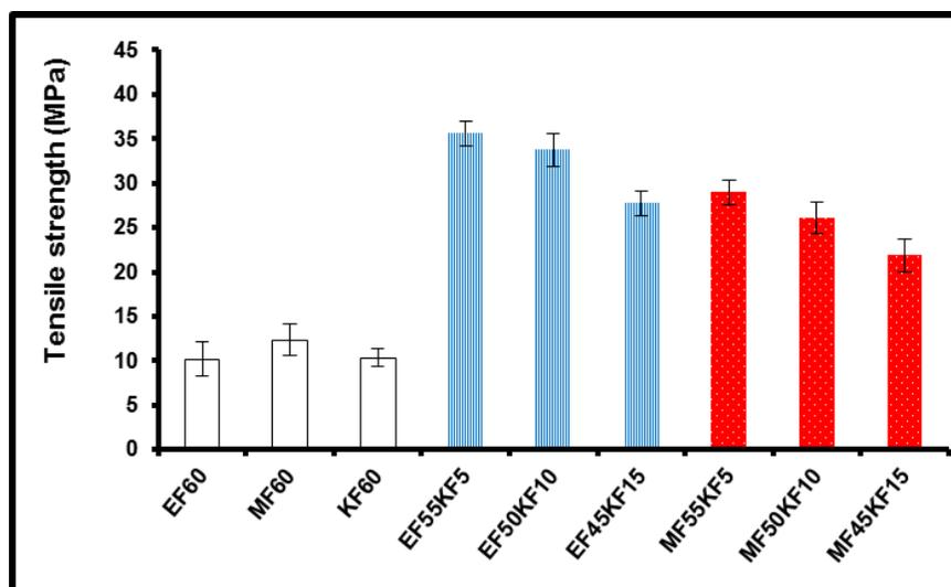
Fig. 4. Tensile strength of hybrid fiber-PLA composites
