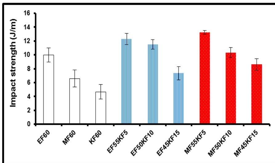
Fig. 9. Impact strength of the hybrid fiber-PLA composites
