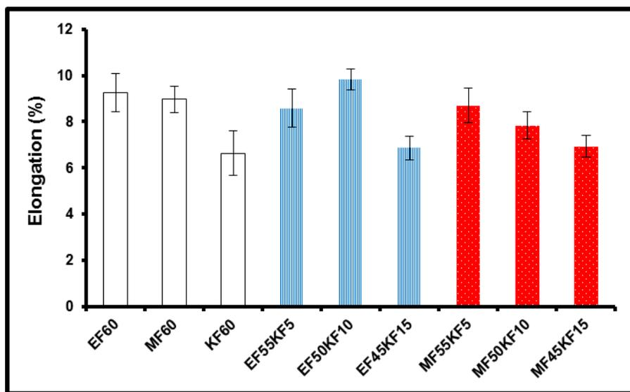
Fig. 6. Elongation at break of hybrid fiber-PLA composites
