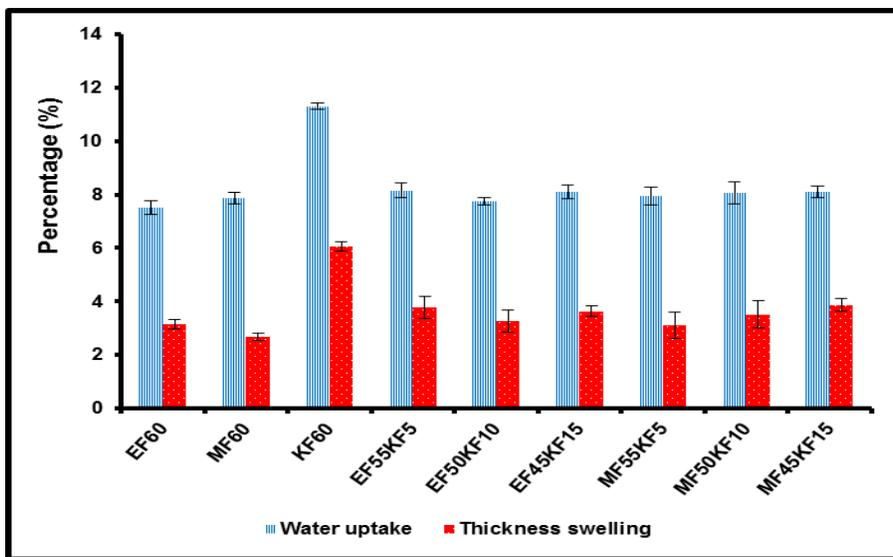
Fig. 11. Dimensional stability of hybrid fiber-PLA composites
