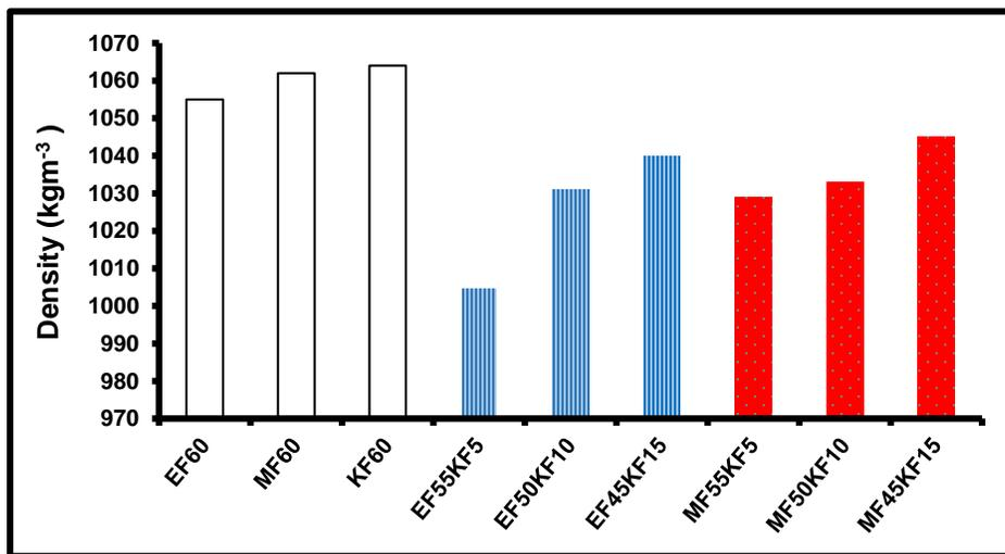
Fig. 10. Density of the hybrid fiber-PLA composites
