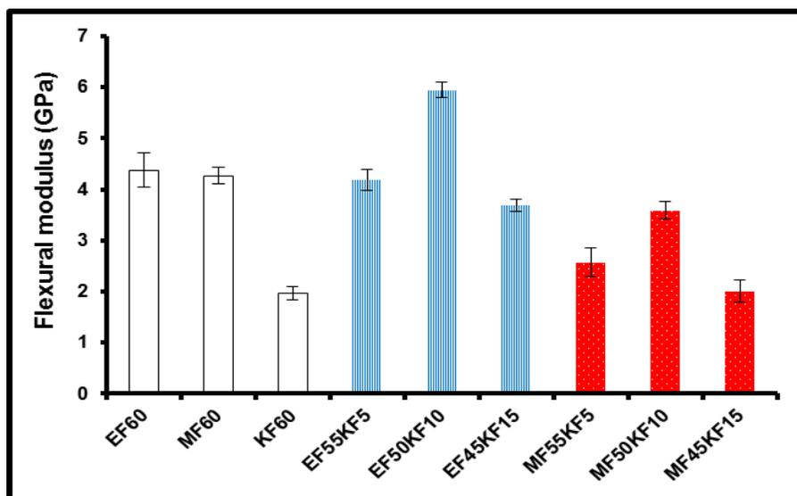
Fig. 8. Flexural modulus of hybrid fiber-PLA composites
