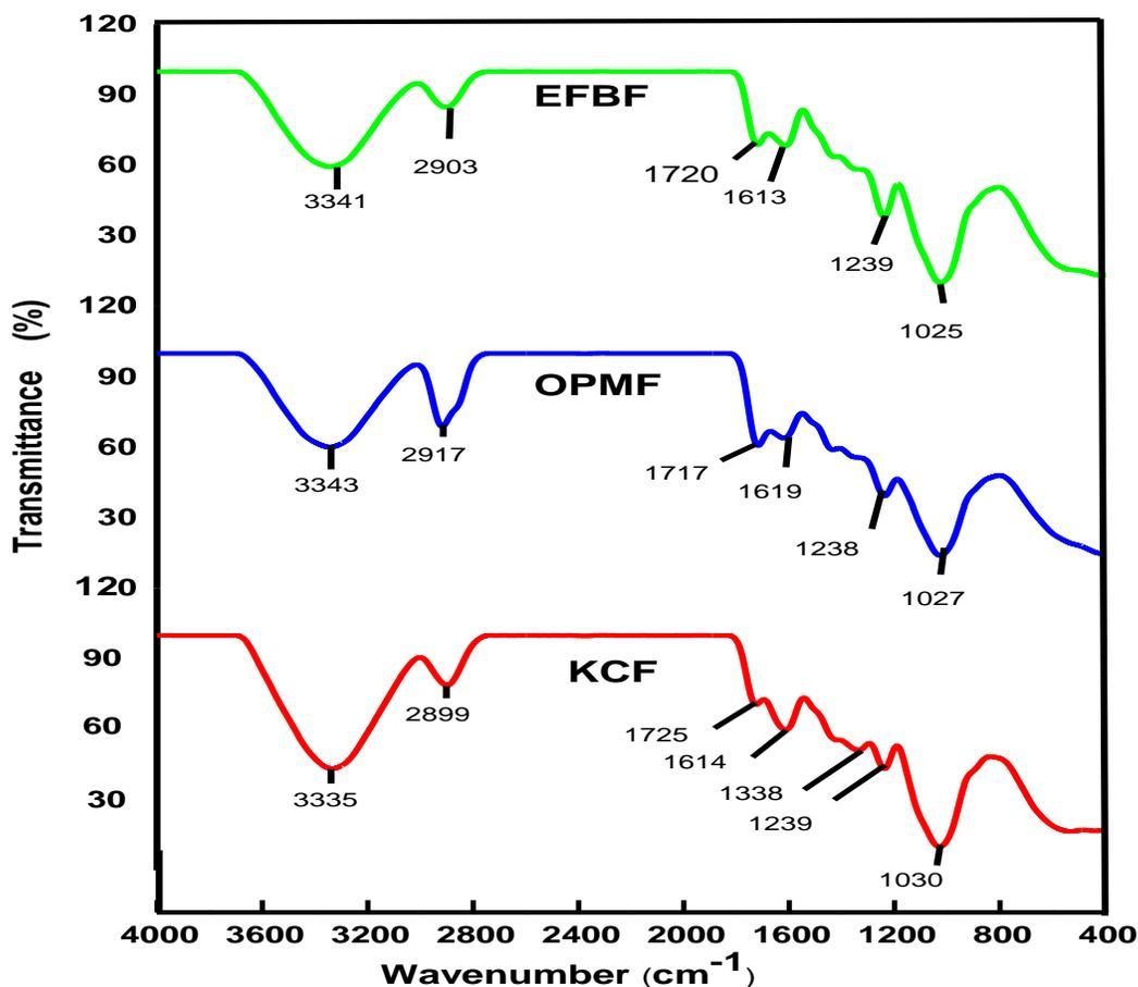
Fig. 12. Fourier transform infrared spectroscopy of pure fibers
