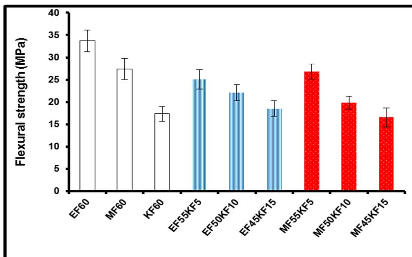
Fig. 7. Flexural strength of hybrid fiber-PLA composites
