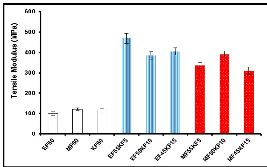
Fig. 5. Tensile modulus of hybrid fiber-PLA composites
