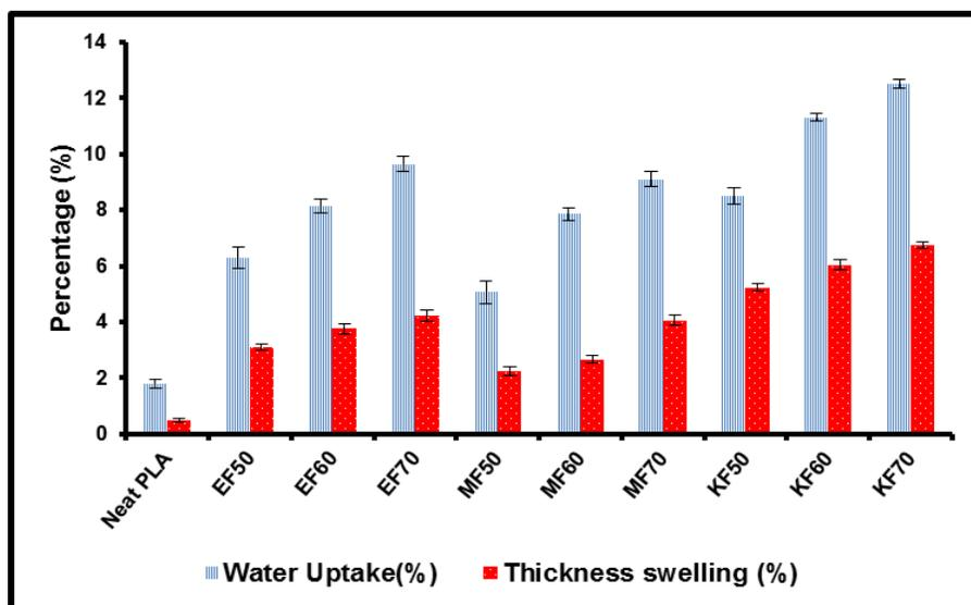
Fig. 3. Dimensional stability of single fiber-PLA composites
