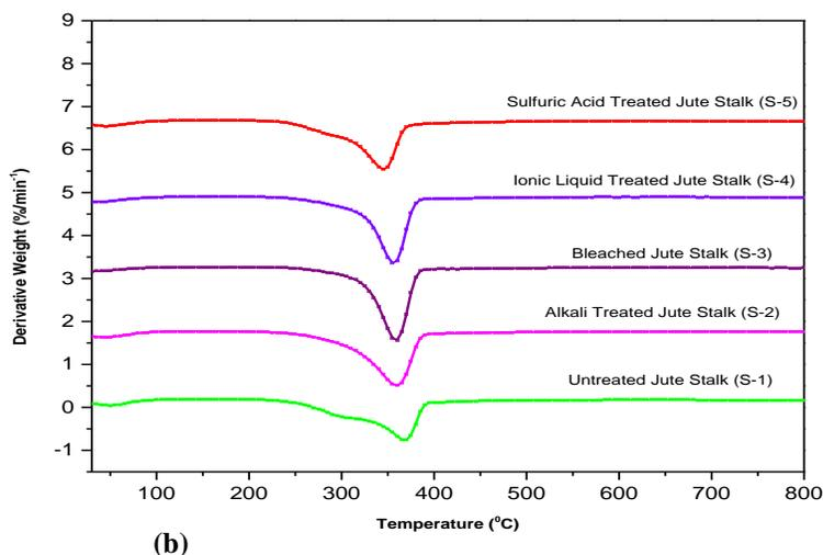
**Fig. 4(b).** DTG spectra for untreated jute stalk (S-1); microwave-assisted alkali-treated jute stalk (S-2); bleached jute stalk (S-3); ionic liquid ([EMIM]<sup>+</sup>Cl<sup>-</sup>) treated jute stalk (S-4); and sulfuric acid (H<sub>2</sub>SO<sub>4</sub>) treated jute stalk (S-5)
