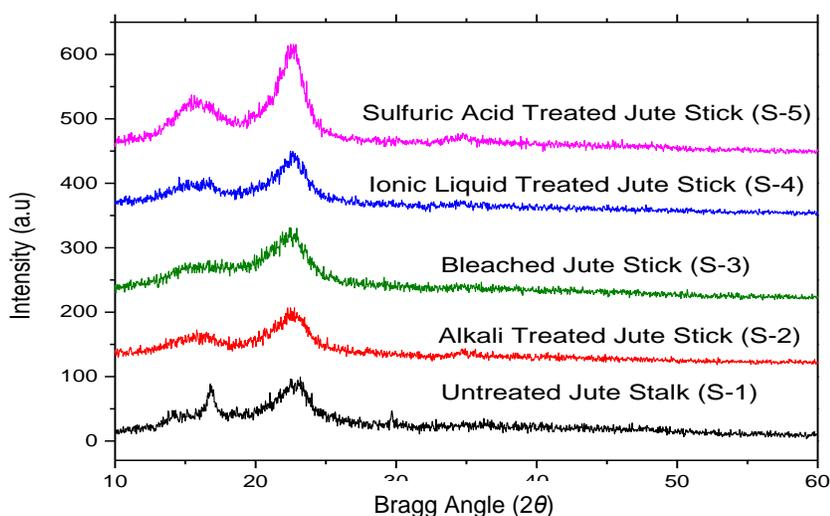
**Fig. 3.** XRD Diffraction of (a) untreated jute stalk (S-1); (b) microwave-assisted alkali-pretreated jute stalk (S-2); (c) bleached jute stalk (S-3); (d) ionic liquid ( $[\text{EMIM}]^+\text{Cl}^-$ )-hydrolyzed jute stalk (S-4); and (e) sulfuric acid ( $\text{H}_2\text{SO}_4$ ) hydrolyzed jute stalk (S-5)
