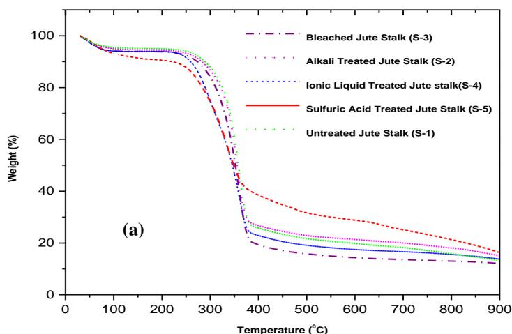
**Fig. 4(a).** TGA spectra for untreated jute stalk (S-1); microwave-assisted alkali-treated jute stalk (S-2); bleached jute stalk (S-3); ionic liquid ([EMIM]<sup>+</sup>Cl<sup>-</sup>) treated jute stalk (S-4); and sulfuric acid (H<sub>2</sub>SO<sub>4</sub>) treated jute stalk (S-5)
