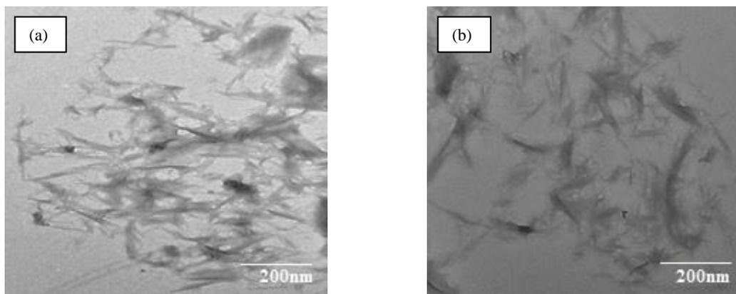
**Fig. 2.** TEM images of (a) Ionic liquid ( $[\text{EMIM}]^+\text{Cl}^-$ ) treated jute stalk (S-4); and (b) sulfuric acid ( $\text{H}_2\text{SO}_4$ ) treated jute stalk (S-5)
