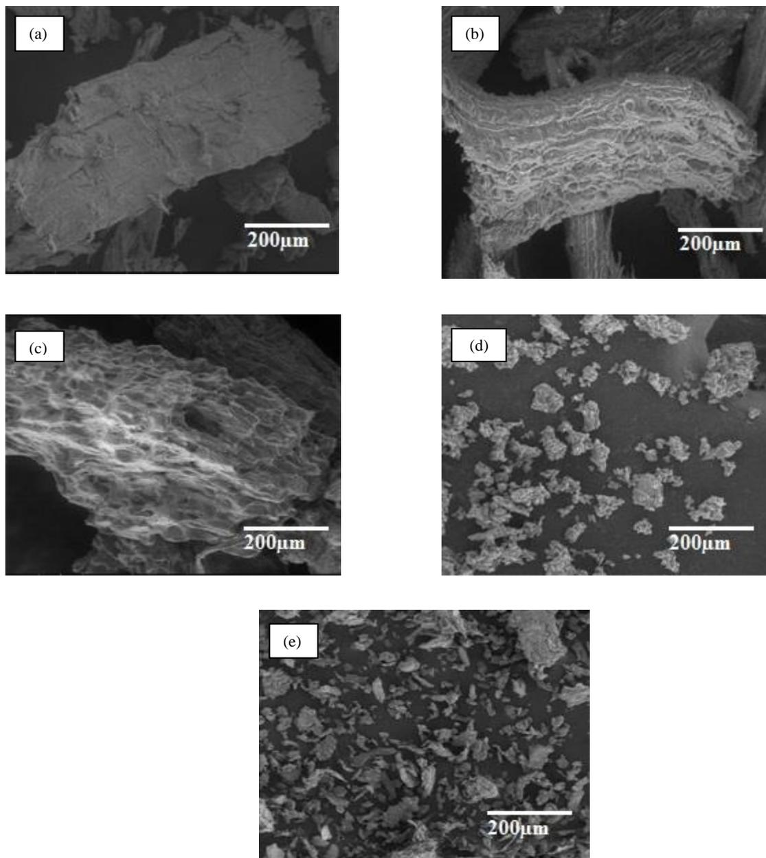
**Fig. 1.** SEM images of (a) untreated jute stalk (S-1); (b) microwave-assisted alkaline-treated jute stalk (S-2); (c) bleached jute stalk (S-3); (d) ionic liquid ([EMIM]<sup>+</sup>Cl<sup>-</sup>) treated jute stalk (S-4); and (e) sulfuric acid (H<sub>2</sub>SO<sub>4</sub>) treated jute stalk (S-5)
