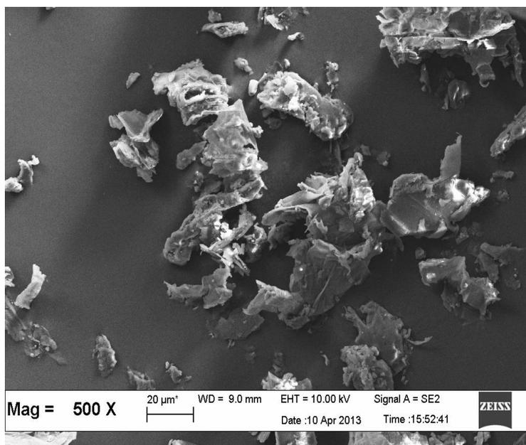
**Fig. 3.** SEM micrograph of the irregular morphology of peanut shell powder
