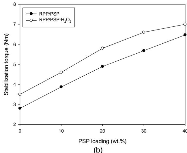
**Fig. 1.** (a) The processing torque of RPP/PSP/H<sub>2</sub>O<sub>2</sub> composites during the 12 min of mixing, and (b) the stabilization torque of RPP/PSP and RPP/PSP-H<sub>2</sub>O<sub>2</sub> composites at different filler loadings
