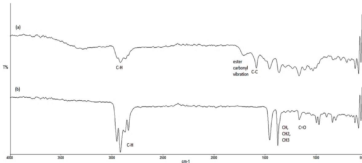
Fig. 4. IR spectra of (a) RPP/PSP and (b) RPP/PSP-H<sub>2</sub>O<sub>2</sub> composites
