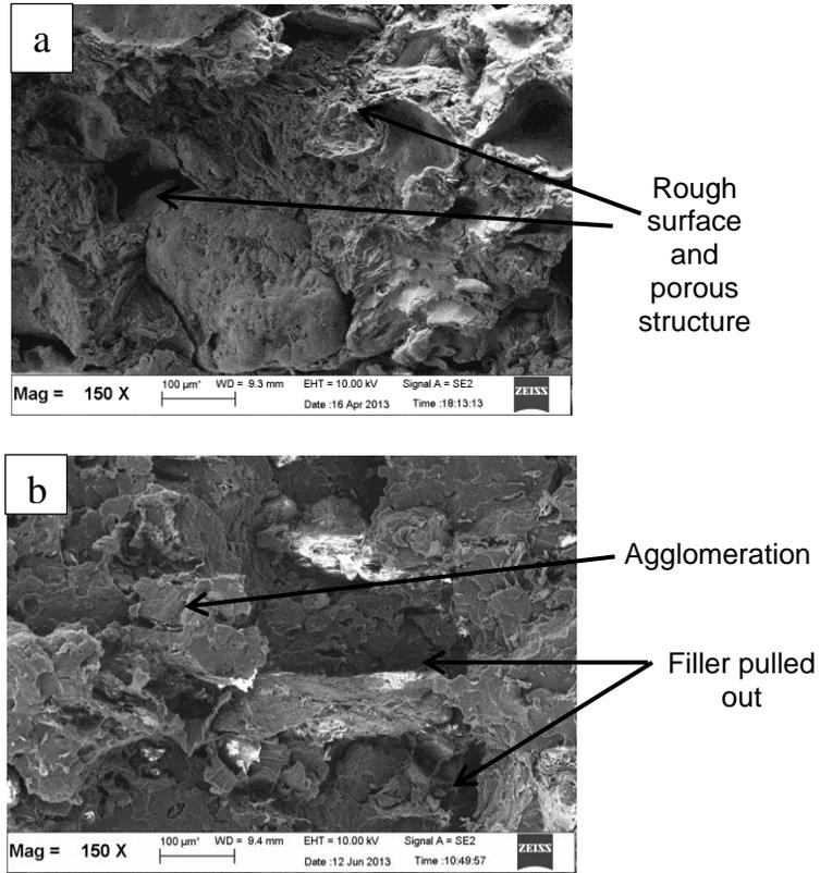
Fig. 5. SEM micrographs of RPP/PSP composites at (a) 10% and (b) 40% filler loading
