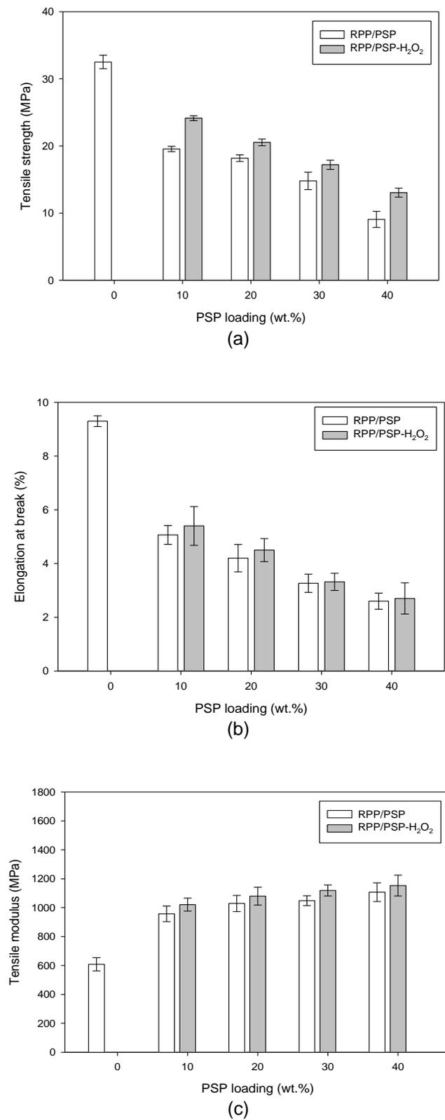
**Fig. 2.** (a) Tensile strength, (b) elongation at break, and (c) tensile modulus of RPP/PSP and RPP/PSP-H<sub>2</sub>O<sub>2</sub> composites at different filler loadings
