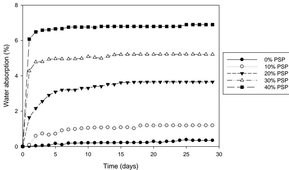
Fig. 7. Water absorption over 30 days of RPP/PSP-H<sub>2</sub>O<sub>2</sub> at different filler loadings
