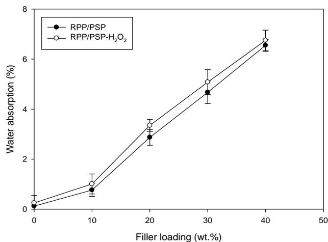
Fig. 8. Equilibrium water absorption of RPP/PSP and RPP/PSP-H<sub>2</sub>O<sub>2</sub> composites at 30 days
