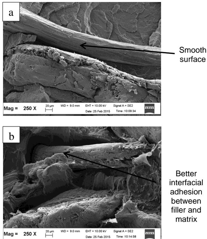
Fig. 6. SEM micrographs of RPP/PSP-H<sub>2</sub>O<sub>2</sub> composites at (a) 10% and (b) 40% filler loading
