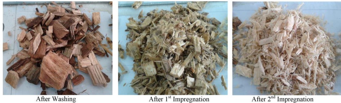
Fig. 2. Chips after washing and the first and second stages of impregnation
