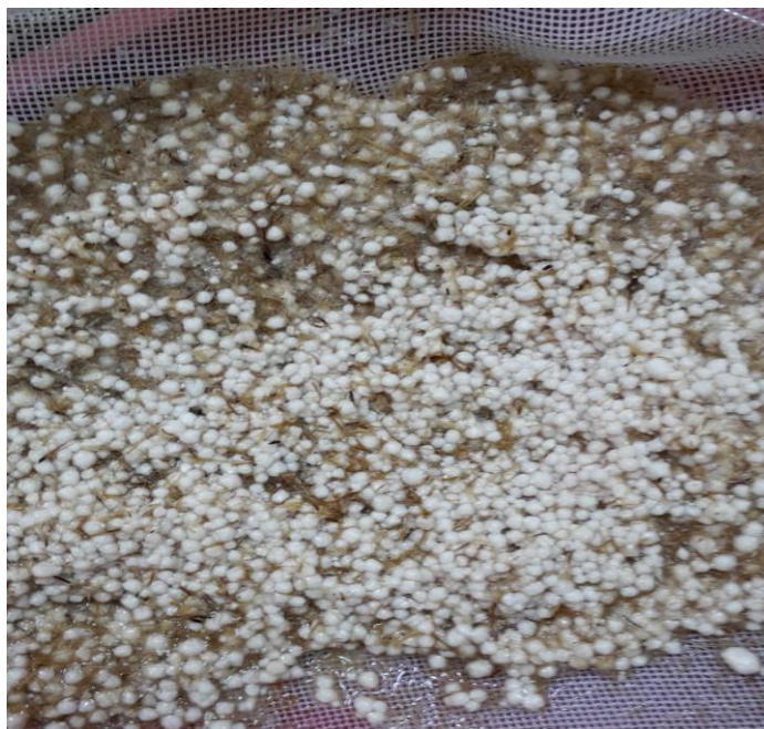
Fig. 7. Solid residues of unconverted substrate and pellet, R. oryzae (NRRL 395)
