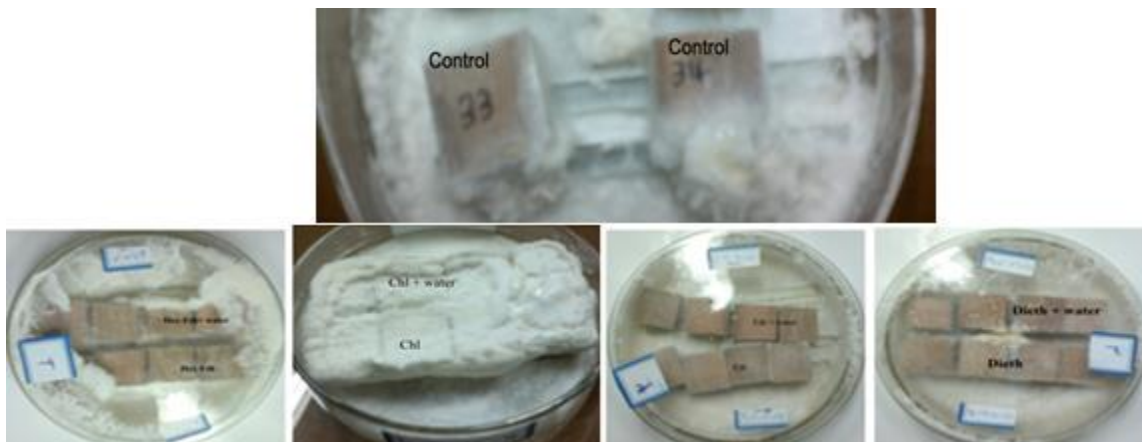
Fig. 1. Mycelium growth of T. versicolor fungus in the extracted samples with different groups of solvents
