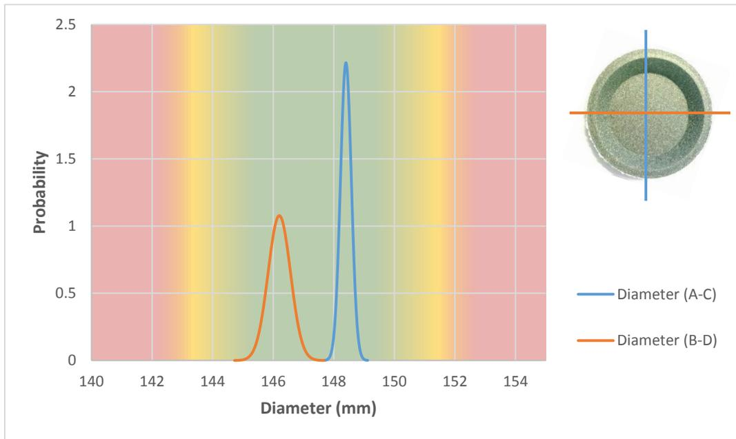
**Fig. 8.** Normal distribution diagram for deformation assessment. The A-C diameter, the predominant fiber direction based on extrusion direction, clearly longer than the B-D diameter. Color gradient in the background describes the preliminary level of acceptance of the product quality of the sample product, where green is Class A product, yellow is Class B product, and red is unacceptable product.
