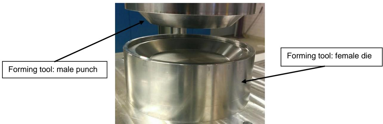
**Fig. 2.** Punch and die tools used for the forming test
