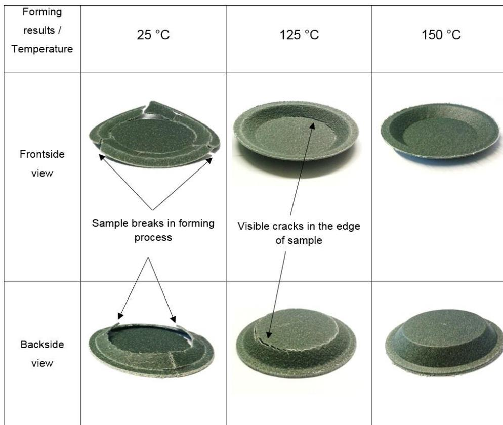
**Fig. 3.** Preliminary forming result. Increasing the temperature of the material before forming resulted in improvement of forming quality (Material breaks in forming at 25 °C, formability improves at 125 °C but the material cracks at angles, forming quality increases with no sign of cracking in 150 °C).
