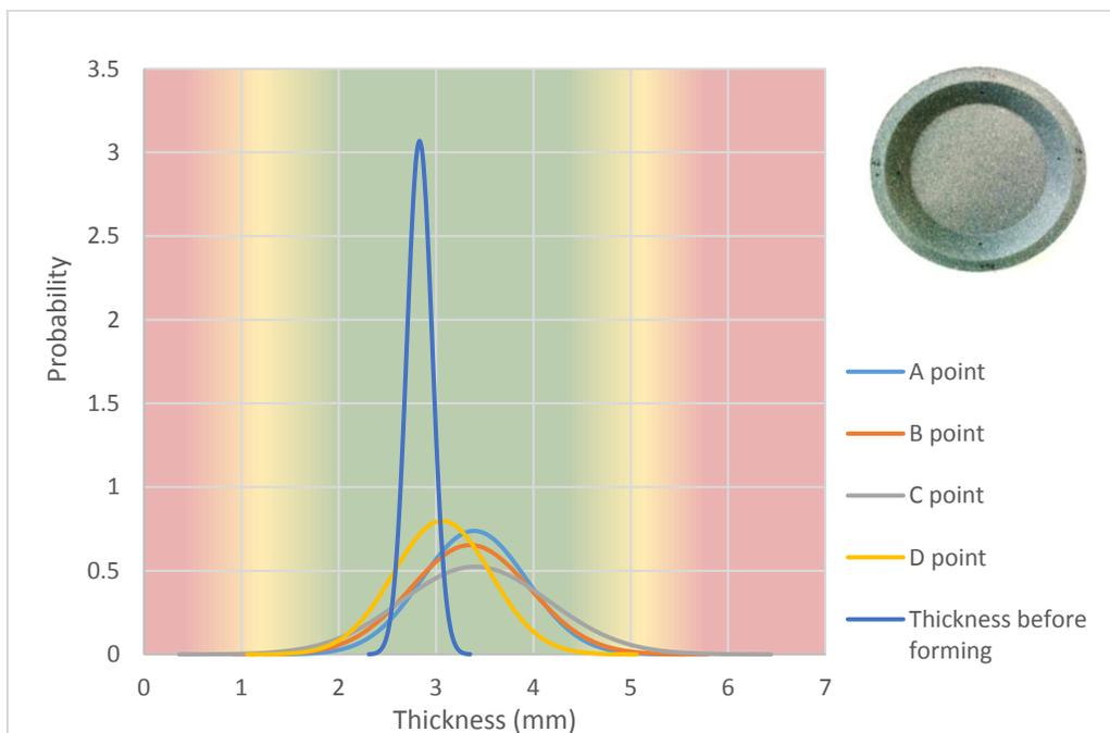
**Fig. 11.** Normal distribution diagram for thickness variation of the tapered section based on four measured points compared to thickness variation of the original sheet. Thickness variation in the original sheet is much lower than thickness variation in the tapered section. Color gradient in the background describes the preliminary level of acceptance range based on durability and corner geometry, where green is Class A product, yellow is Class B product, and red is an unacceptable level.
