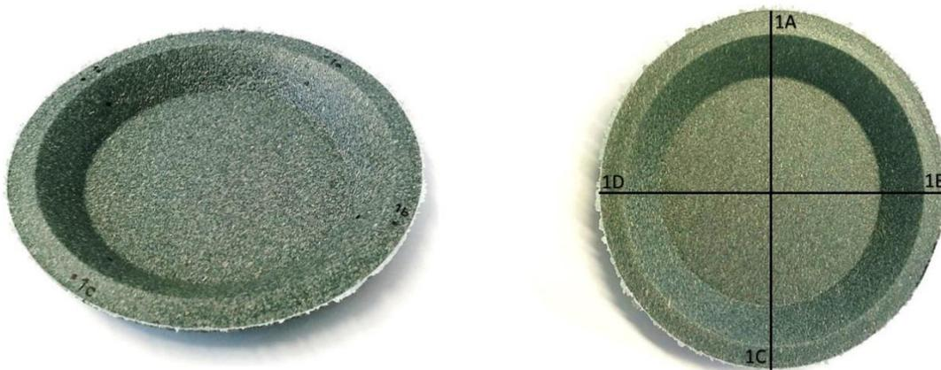
**Fig. 6.** Sample #1 and divided sections A-D used for shape deformation and thickness variation measurement
