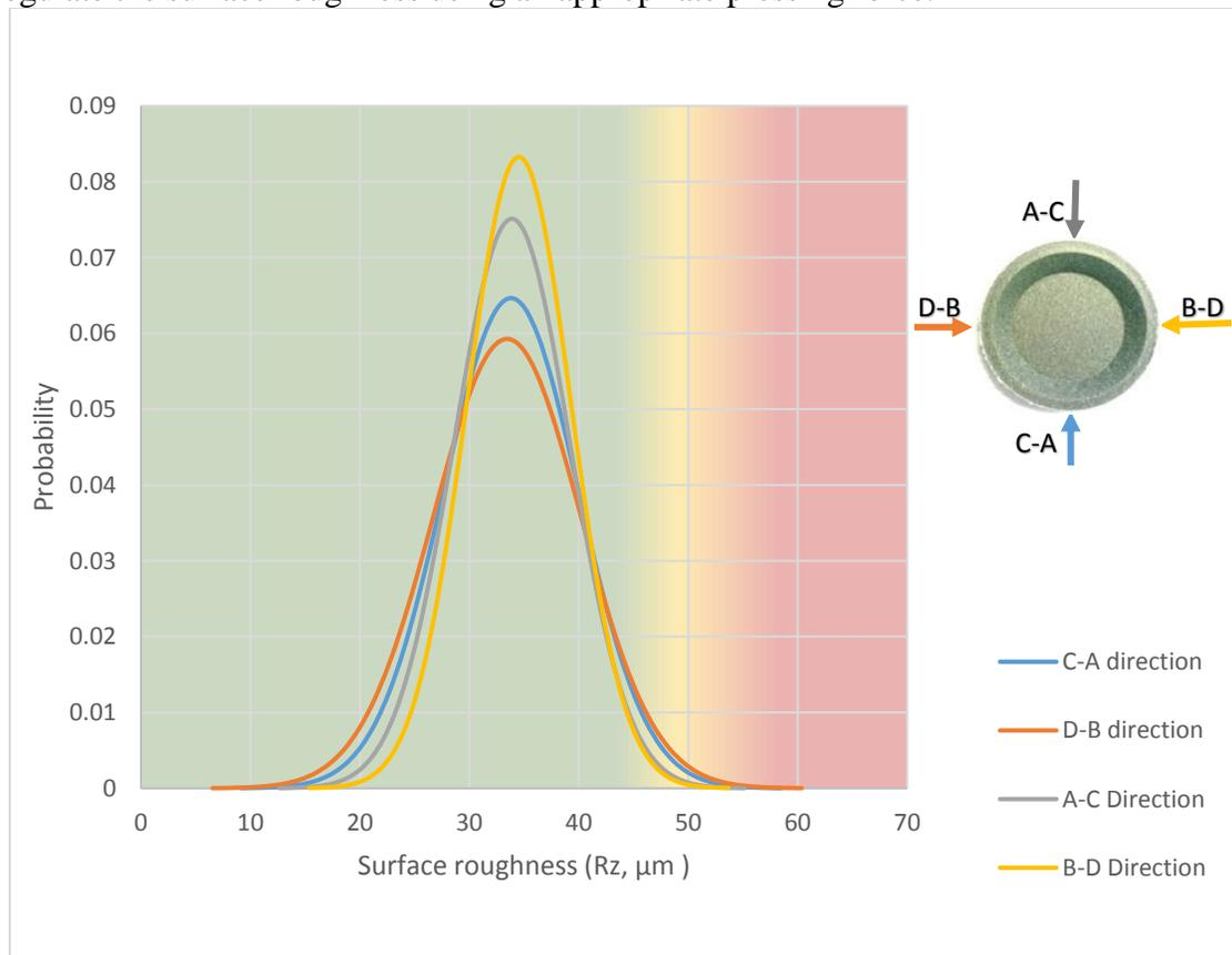
**Fig. 9.** Normal distribution diagram for surface roughness measurement based on four measured sections. Roughness variation in the A-C direction (extrusion direction) was less than in the B-D direction. Color gradient in the background describes the preliminary level of acceptance range based on visual and tactile inspection, where green is Class A product, yellow is Class B product, and red is unacceptable level.
