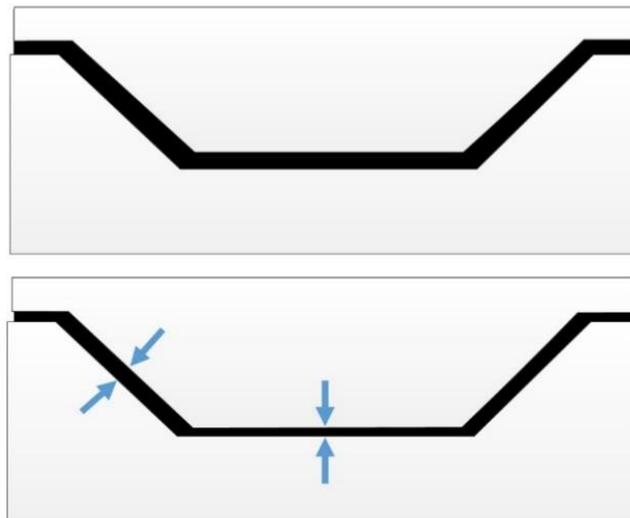
**Fig. 12.** Effects of tool forming tolerance on material thickness variation. The highlighted areas in the lower image present thickness variation of the material in the process caused by forming tools while the upper image shows constant thickness.
