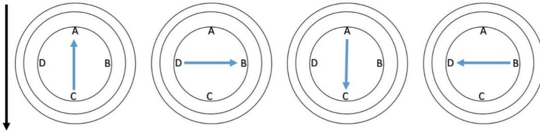
**Fig. 7.** Four directions measured in the surface roughness test. All samples were divided in four sections such that the A-C direction is the extrusion direction of the plates.
