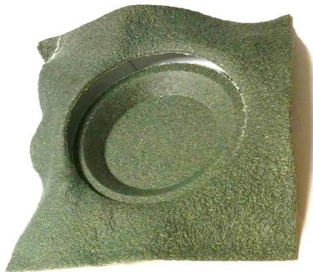
**Fig. 4.** Sample plate before detaching of the product from the WPC sheet
