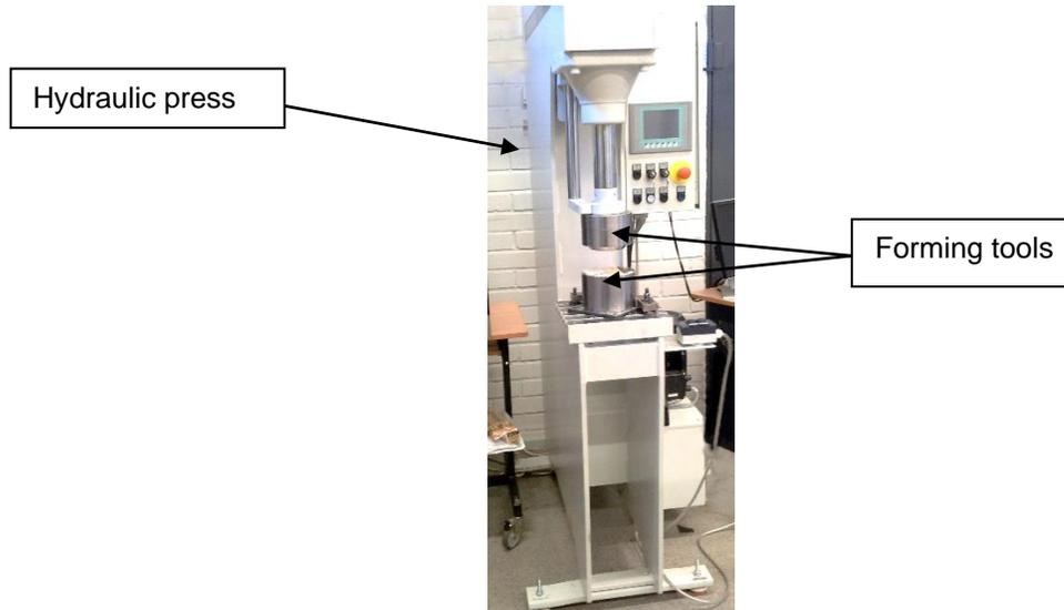
**Fig. 1.** Pressing tools mounted on the hydraulic press
