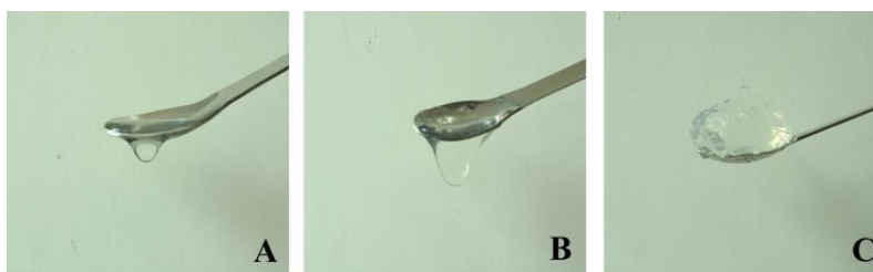
Fig. 3. Pictures of three different NFC suspensions: (A) 0.8 wt% NFC, (B) 1.2 wt% NFC, (C) 3.0 wt% NFC
