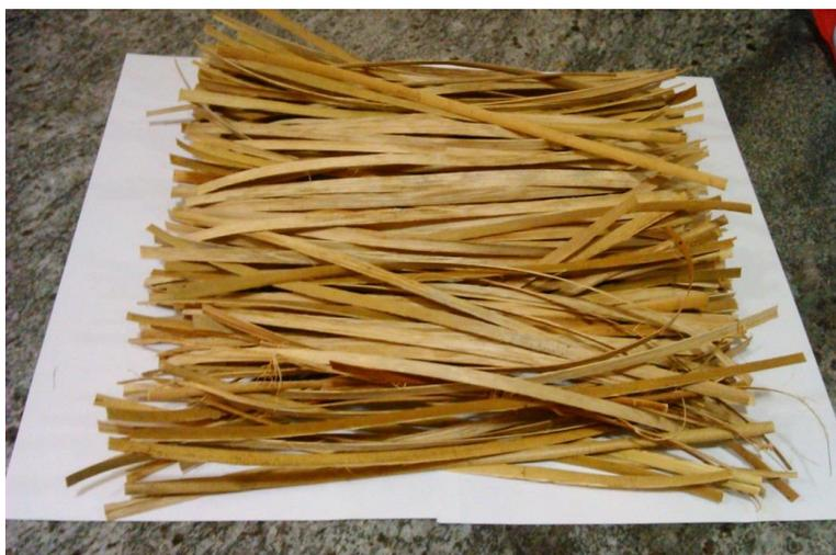
**Fig. 1.** Extracted raw fibers of leaf stalk
