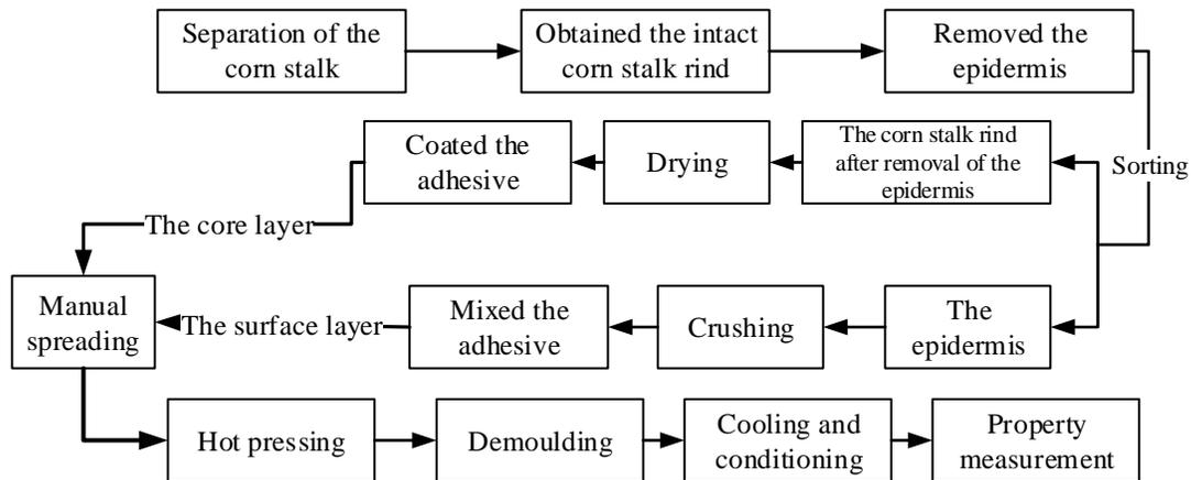
**Fig. 1.** Process for manufacturing composite board from corn stalk rinds
