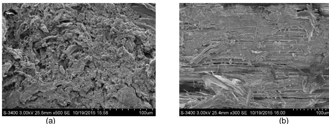
Fig. 5. Microscopic observation of (a) the surface layer (500X) and (b) the core layer (300X)
