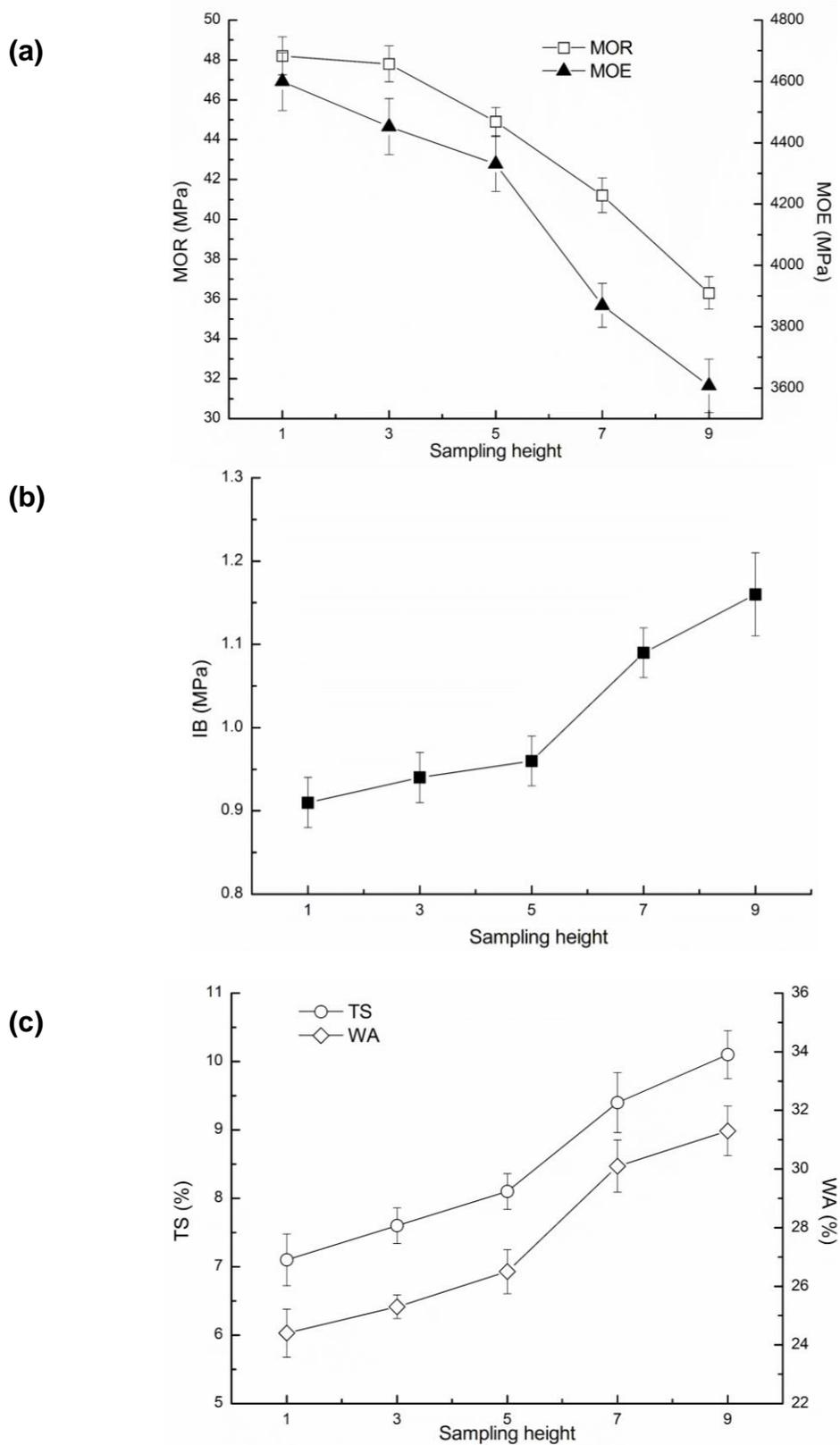
**Fig. 3.** Effect of sampling height on corn stalk rind composite (a) MOR and MOE; (b) IB; and (c) TS and WA. The numbers 1, 3, 5, 7, and 9 indicate the root, bottom, ear, top half, and top part of the corn stalk rind, respectively.
