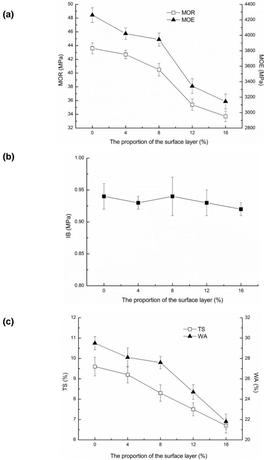
**Fig. 4.** Effect of surface layer proportion on corn stalk rind composite board (a) MOR and MOE; (b) IB; and (c) TS and WA
