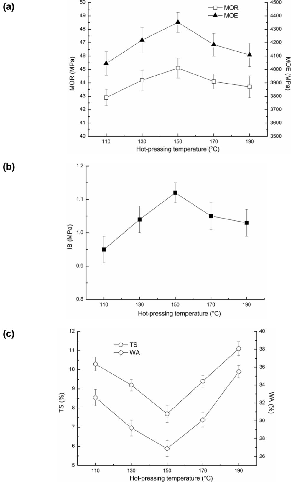
**Fig. 6.** Effect of the hot-pressing temperature on the on corn stalk rind composite board (a) MOR and MOE; (b) IB; and (c) TS and WA
