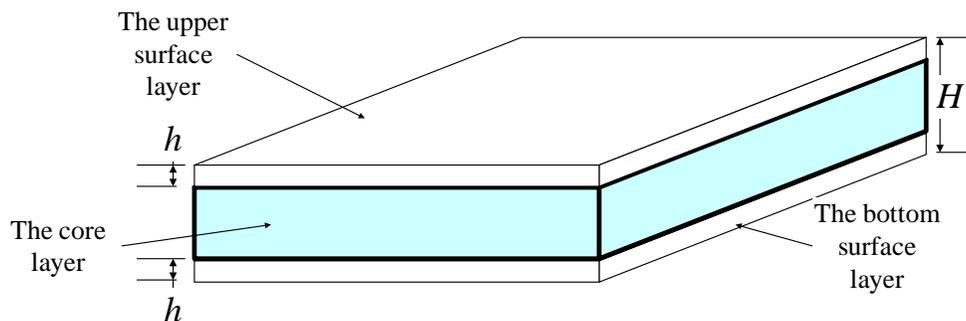
**Fig. 2.** Structure of the corn stalk rind composite board
