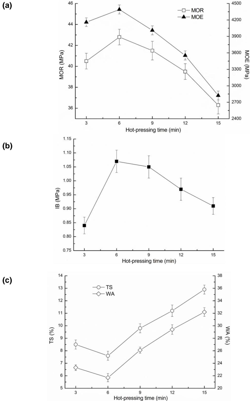
**Fig. 7.** Effect of the hot-pressing time on corn stalk rind composite board (a) MOR and MOE; (b) IB; and (c) TS and WA
