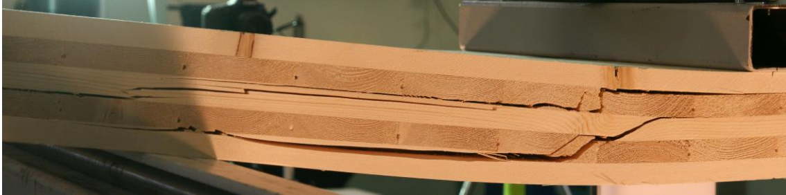
Fig. 11. Failure due to a combination of longitudinal shear and initial rolling shear near to the bondlines
