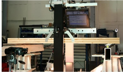
Fig. 5. Four point bending test of CLT panels with an alternating layer configuration
