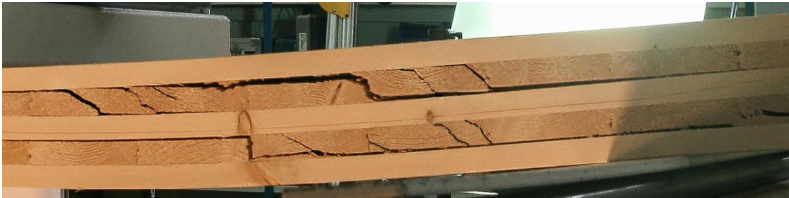
Fig. 9. Failure due to initial rolling shear near to bondlines appeared as shear stress transverse to the grain
