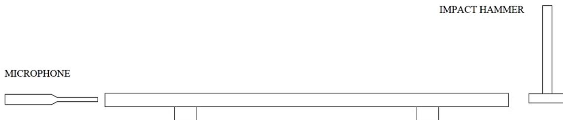
**Fig. 3.** The principle of longitudinal vibration method
