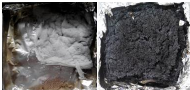
Fig. 5. Macro-morphology of untreated (left) and treated (right) ULDFs viewed using a common digital camera
