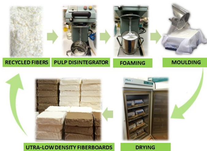
Fig. 2. Preparation process for ultra-low density fibreboard
