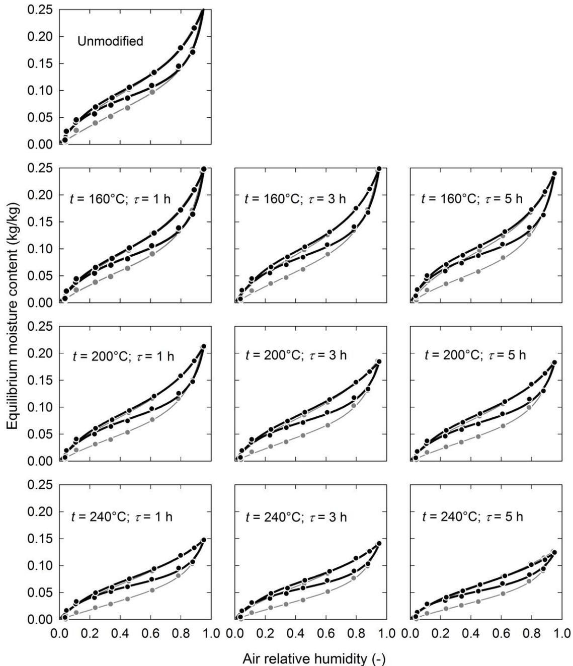
**Fig. 1.** The equilibrium moisture content (dots) and modeled sorption isotherms (curves) of thermally treated spruce wood. Black curves, after cyclic sorption; gray curves, before cyclic sorption
