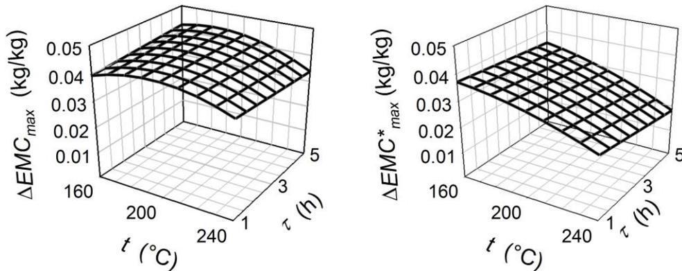
**Fig. 4.** Response surface model of maximum difference of equilibrium moisture content as a function of thermal treatment temperature and time before (left) and after (right) cyclic sorption
