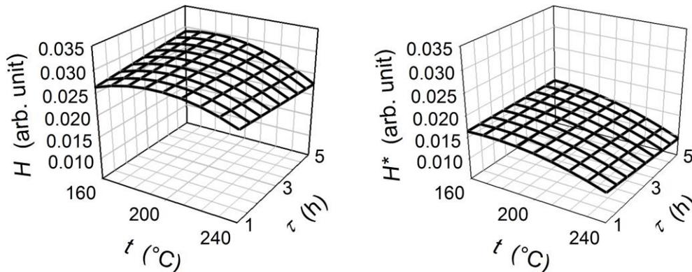
**Fig. 3.** Response surface model of hysteresis loop as a function of treatment temperature and time before (left) and after (right) cyclic sorption
