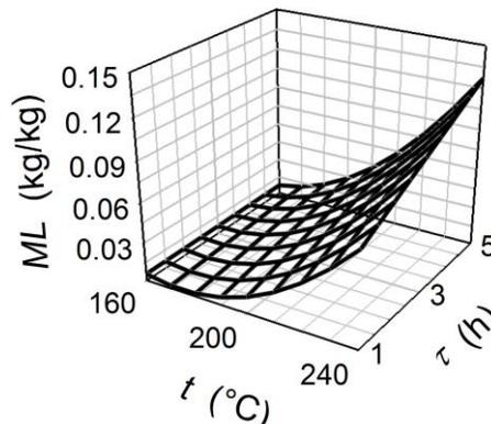
**Fig. 2.** Response surface model of mass loss as a function of treatment temperature and time
