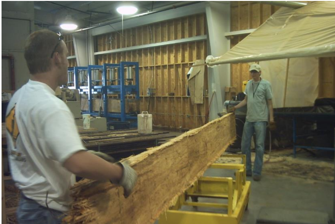
Fig. 1. Typical rough beam shown immediately after pressing
