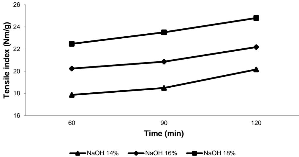
Fig. 1. The effect of condition and duration of cooking on paper tensile indices
