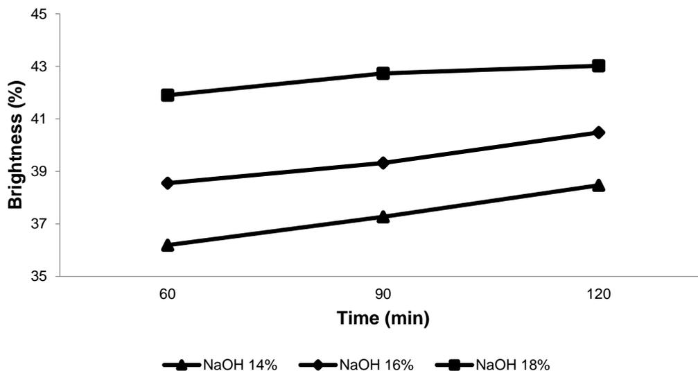
Fig. 5. The effect of condition and duration of cooking on paper brightness
