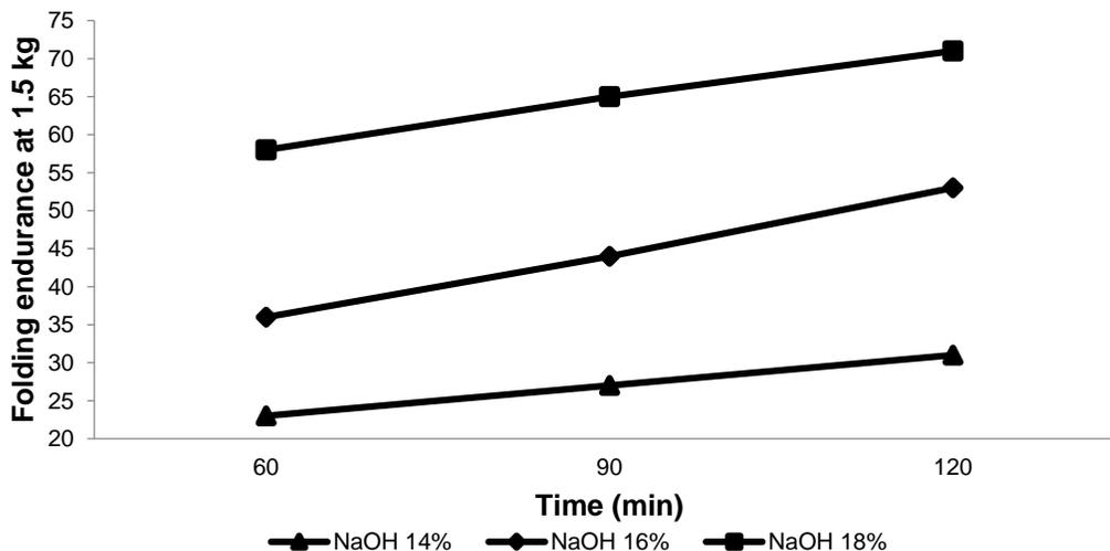
Fig. 4. The effect of condition and duration of cooking on paper folding endurance
