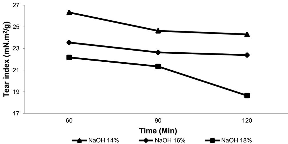
Fig. 2. The effect of condition and duration of cooking on paper tear indices
