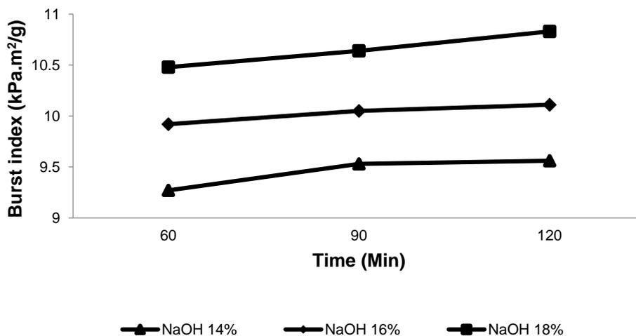
Fig. 3. The effect of condition and duration of cooking on paper burst indices
