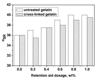
Fig. 10. Drainage performances of untreated gelatin and cross-linked gelatin
