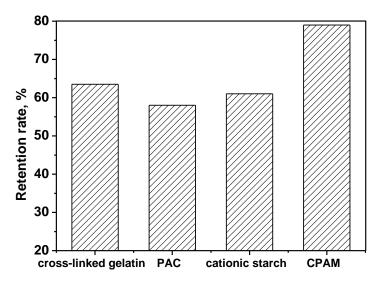
Fig. 6. Comparison of cross-linked gelatin and the commercial retention aids
