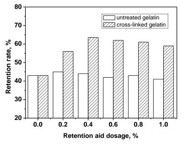
Fig. 5. Retention performances of untreated gelatin and cross-linked gelatin
