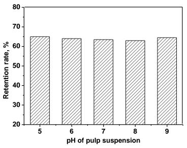
Fig. 8. The effect of pH on the retention performances of cross-linked gelatin
