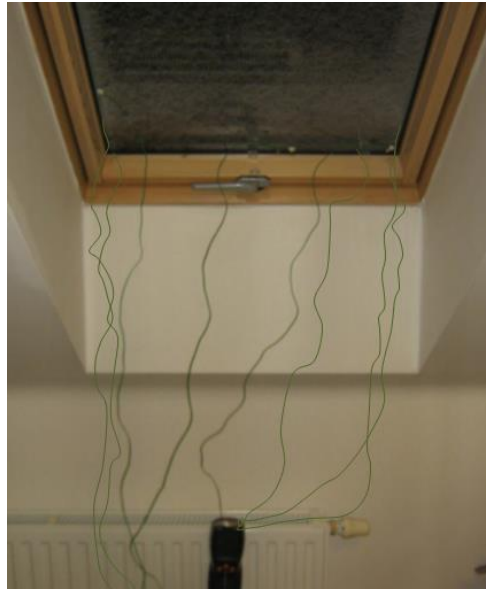
Fig. 3. Positioning of the temperature sensors on the inside of the insulating double glazing in the lower area of the glazing
