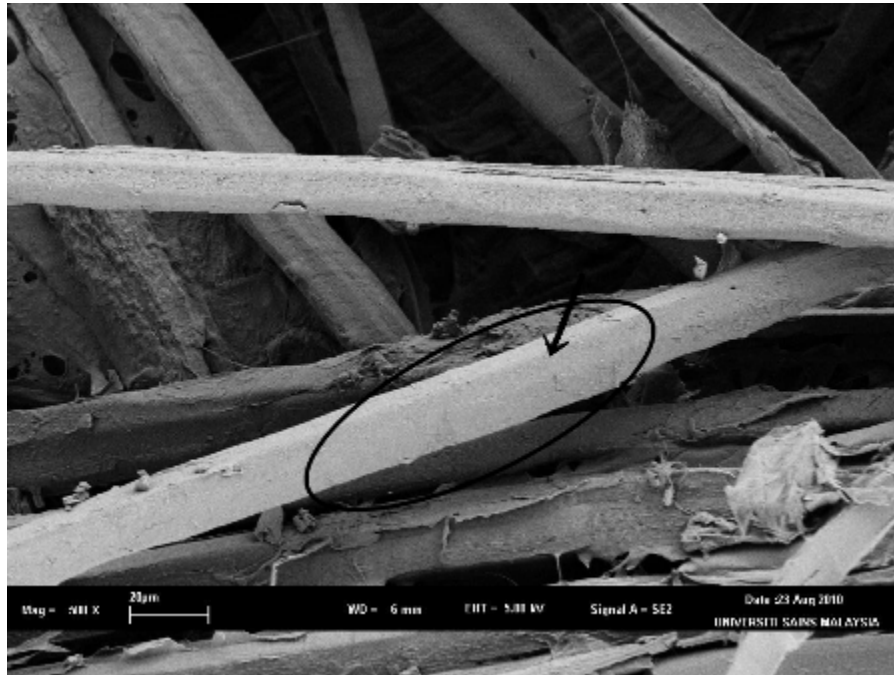
Fig. 7(a). SEM micrograph of succinylated kenaf bast fibres, showing surface of succinylated fibre (x500)
