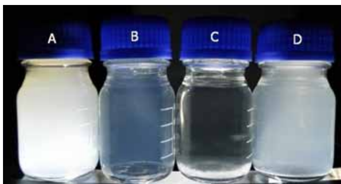
Fig. 5. Appearance images of cellulose nanocrystal suspensions after oxidation (A) and dilution to 0.1%; (B), the oxidized fibers (the water-ratio of that was 0.1%); after treatment by the homogenizer (C) and ultrasound (D)
