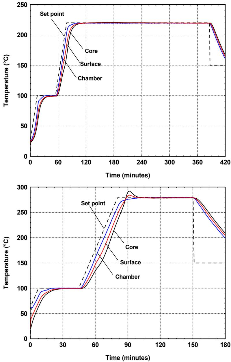
Fig. 1. The temperature evolutions for two contrasted tests (top: 220 °C – 5h and bottom: 280 °C - 1h)
