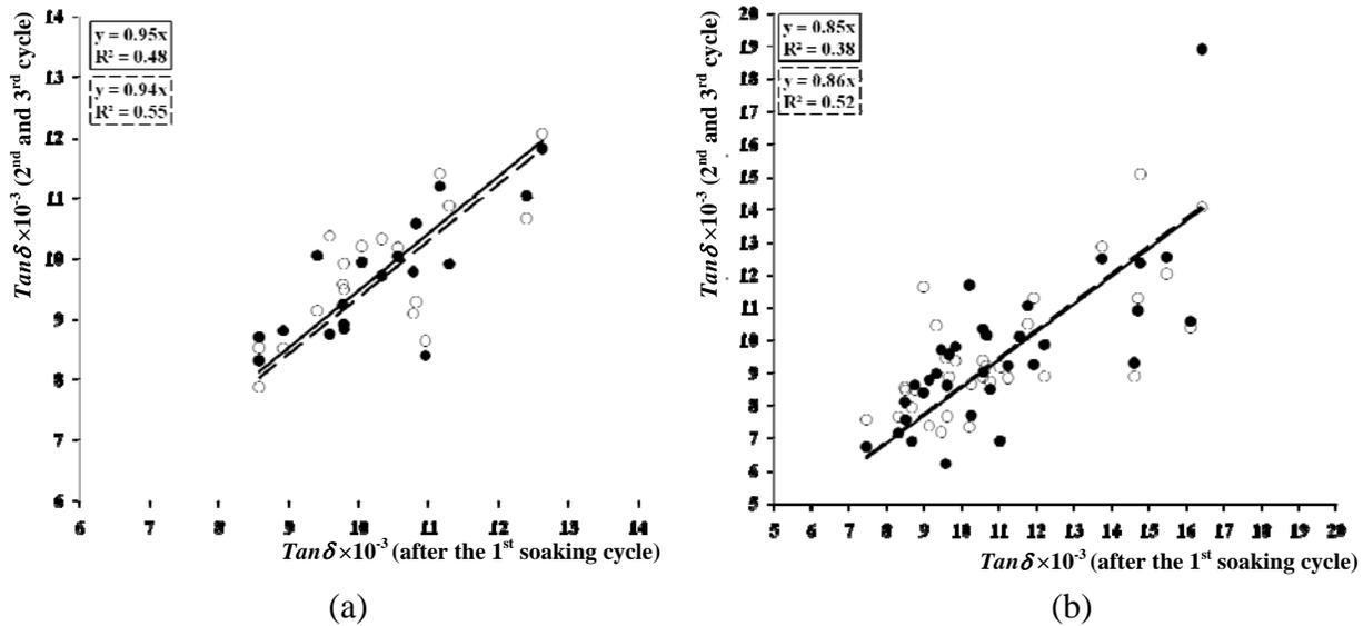
**Fig. 3.** Relationship between damping coefficient  $\tan\delta$  after the first, second and third soaking cycle (a: Mulberry, b: Walnut, o: after the 2<sup>nd</sup> cycle, •: after the 3<sup>rd</sup> cycle)
