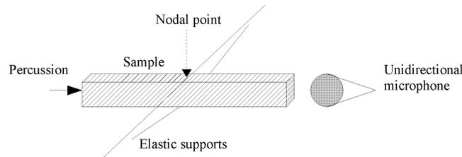
**Fig. 1.** Experimental setup, free-free bar in longitudinal vibration (Inspired from US-Patent 2004/0144158 A1)
