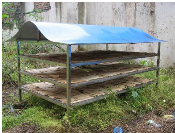
Fig. 2. Shelf employed in the field test
