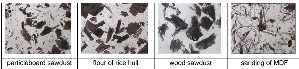
Fig. 1. Microscopic photos of the fillers (4X)
