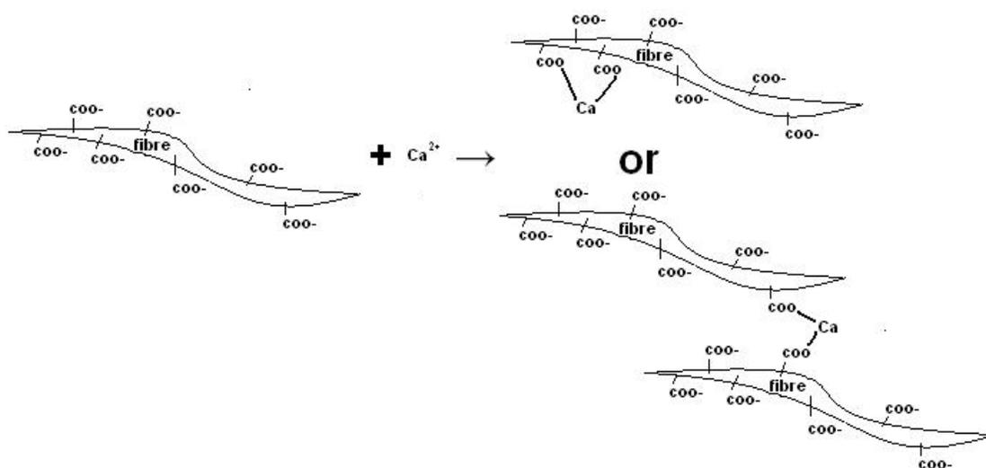
**Fig. 3.** The adsorption model between carboxyl groups and  $\text{Ca}^{2+}$
