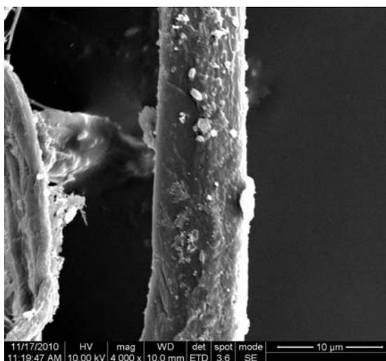
**Fig. 7.** Fibers of bleached eucalyptus pulp with deposits formed by  $\text{Ca}^{2+}$  and DCS model substances
