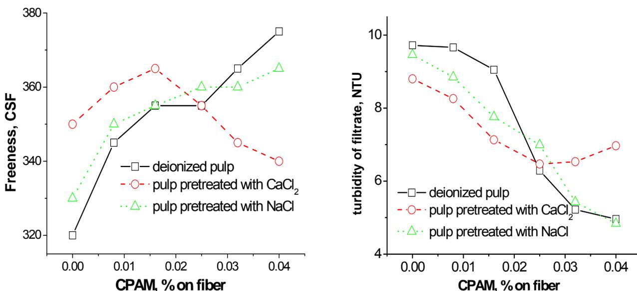
**Fig. 4.** Charge screening effect of  $\text{Ca}^{2+}$  and  $\text{Na}^+$  on CSF of pulp and turbidity of filtrate (conc. of pulp was 0.3% oven-dry, different dosages of CPAM and 0.05%Silica were added sequentially)
