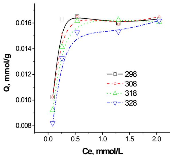
**Fig. 1.** Sorption isotherm of  $\text{Ca}^{2+}$  on deionized kraft pulp from mixture of  $\text{Ca}^{2+}$  and  $\text{Na}^+$  solution at pH 7.5
