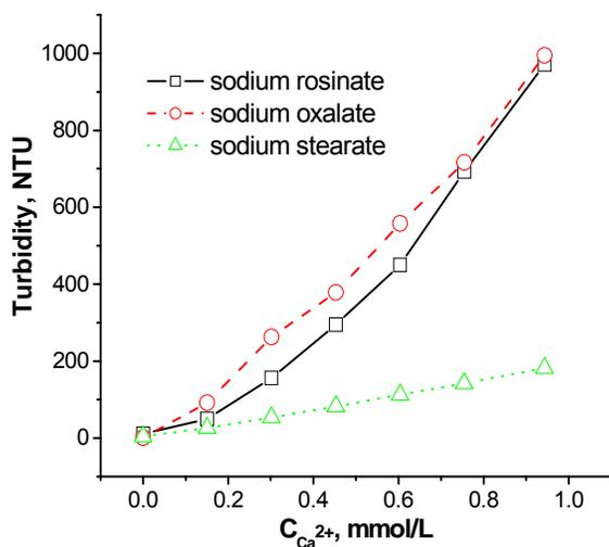
**Fig. 5.** Effect of Ca (II) on the turbidity of DCS model substances solutions
