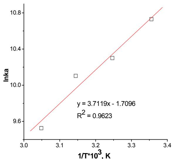
**Fig. 2.** Effect of temperature of  $\text{Ca}^{2+}$  adsorption on hardwood pulp
