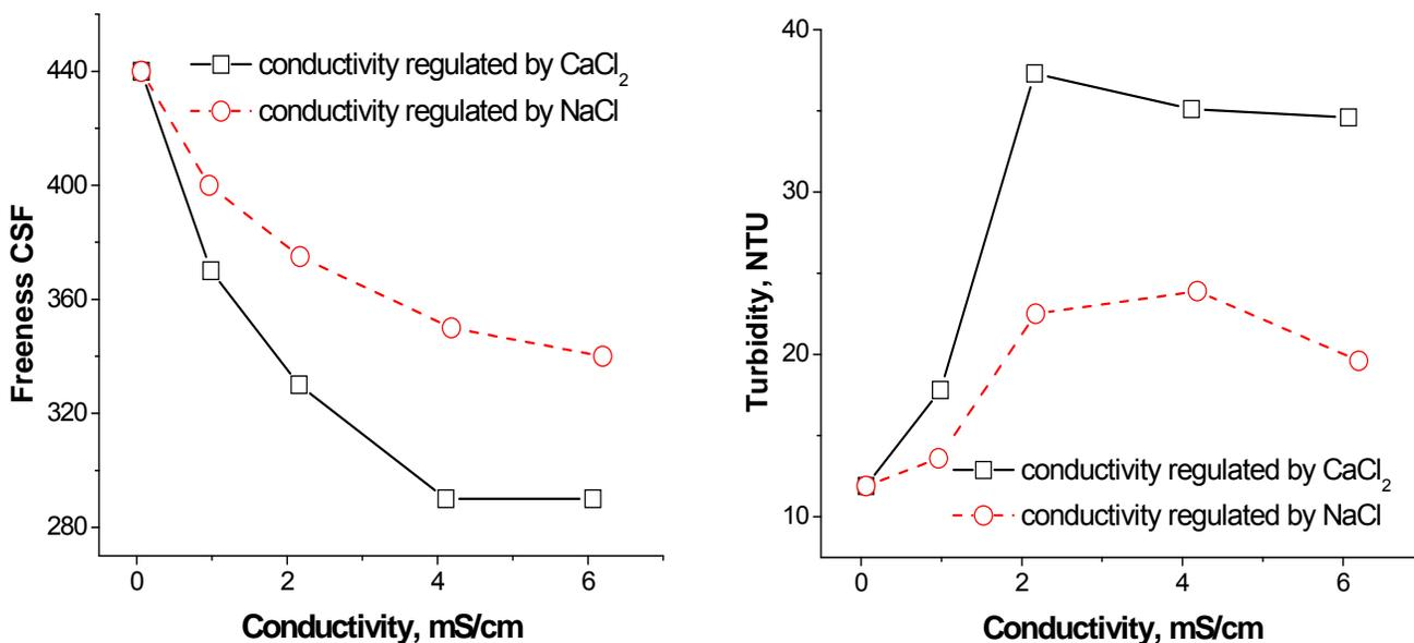
**Fig. 8.** Effect of conc. of  $\text{Ca}^{2+}$  on CSF of pulp and turbidity of filtrate when conc. of DCS was 0.06g/L (conc. of deionized pulp was 0.3% oven-dry, different dosages of  $\text{CaCl}_2$  or NaCl, 0.02% CPAM and 0.05% Silica were added sequentially)
