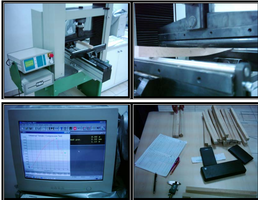
Fig. 4. The bending strength and modulus of elasticity module experiments
