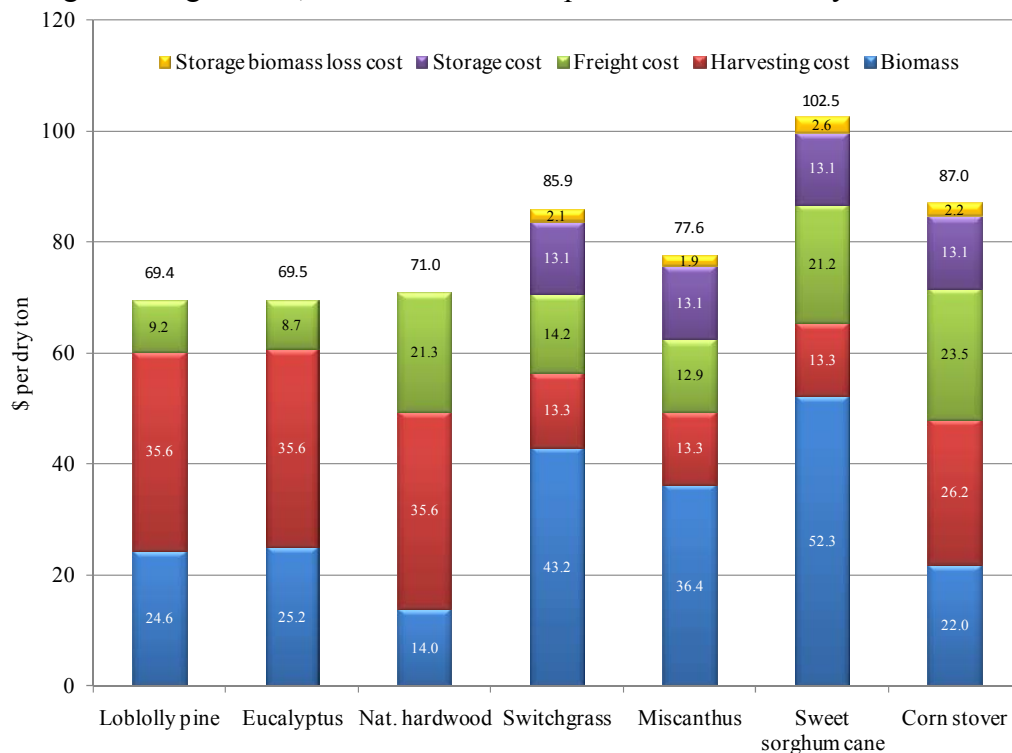
Figure 3. Delivered cost of biomass for each of the feedstock, assuming a 5% covered area and annual supply of 453,597 dry ton year -1
