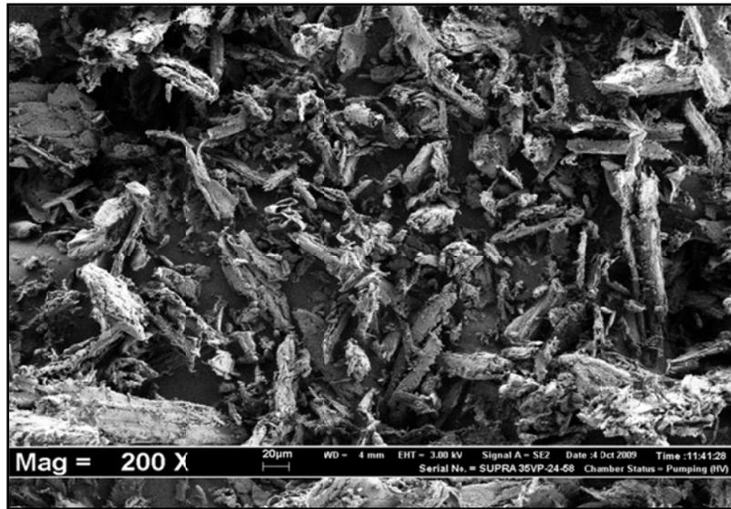
Fig. 4. SEM micrograph of irregular morphology of kenaf powder
