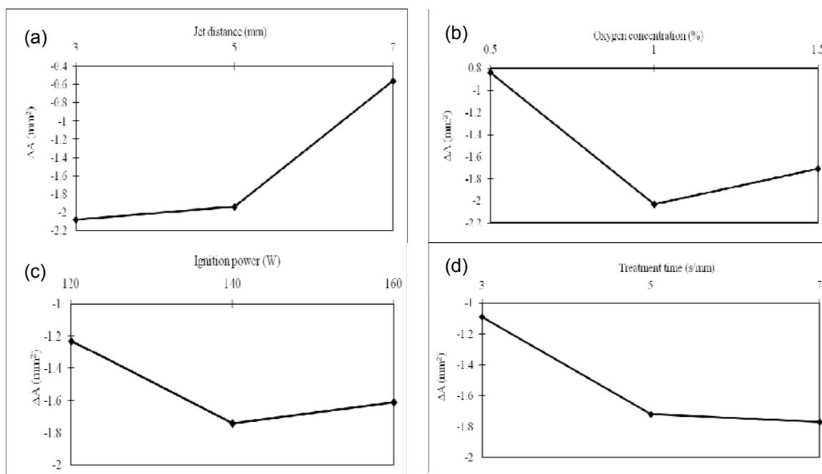
Fig. 6. Statistical trend analysis of reduction of wetted area after  $\text{O}_2$  atmospheric pressure plasma treatment with different parameters: (a) jet distance ( $d$ ), (b) concentration of  $\text{O}_2$  ( $O$ ), (c) ignition power ( $P$ ), and (d) treatment time ( $s/\text{mm}$ ).
