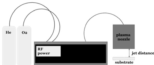
Fig. 1. Schematic diagram of He-O<sub>2</sub> plasma treatment on cotton fabric
