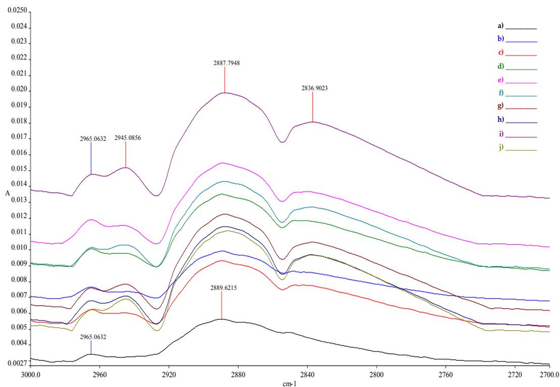
**Fig. 3.** FTIR spectra of oxygen plasma-modified cotton fabrics in the region of 3000-2700  $\text{cm}^{-1}$ . Spectrum (a) represents the control fabric, while spectra (b)-(j) represent the optimisation runs 1-9, respectively.
