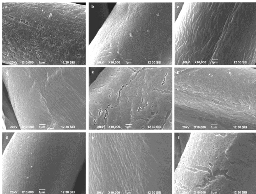
**Fig. 5.** SEM micrographs illustrate surface morphology of cotton fibres exposed to O<sub>2</sub> atmospheric pressure plasma (magnification 10,000x). Micrographs (a)-(i) represent optimisation runs 1-9, respectively.
