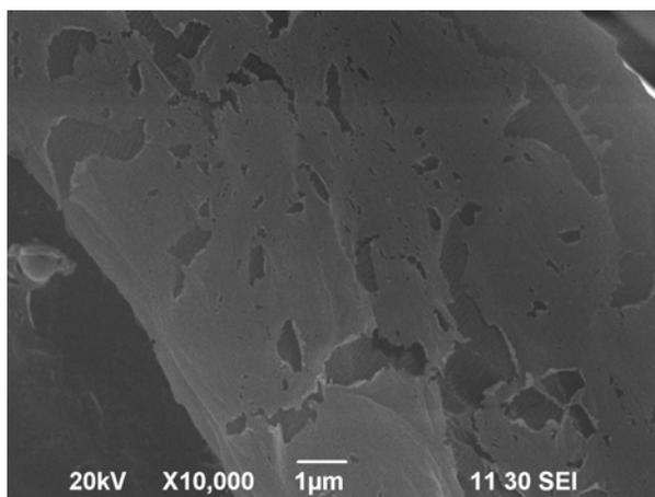
**Fig. 7.** Surface morphology of cotton fibres modified under optimal condition (operation parameters: 3mm, 1% O<sub>2</sub>, 7s/mm and 140W) at 10,000x
