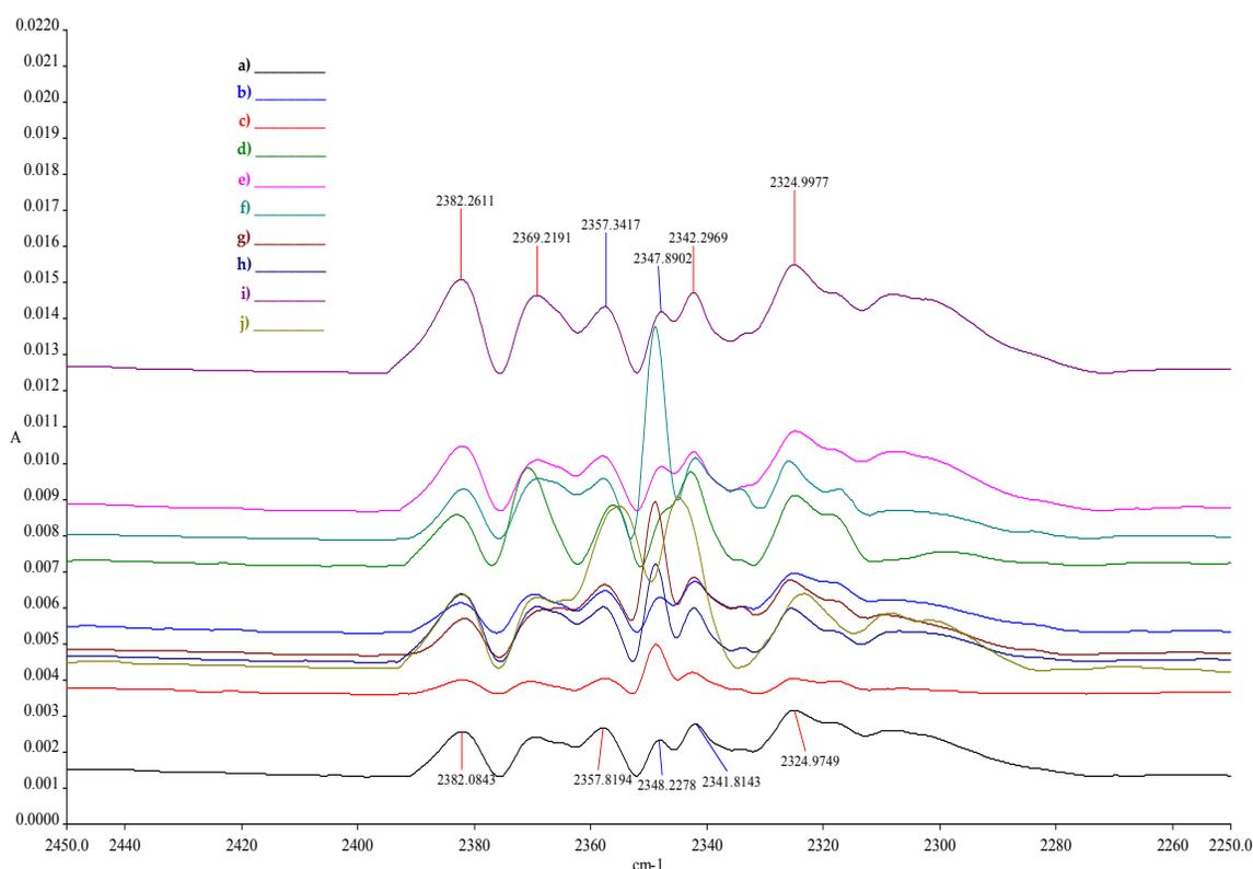
**Fig. 2.** FTIR spectra of oxygen plasma- modified cotton fabrics in the region of  $2400\text{-}2280\text{ cm}^{-1}$ . Spectrum (a) represents the control fabric, while spectra (b)-(j) represent the optimisation runs 1-9, respectively.
