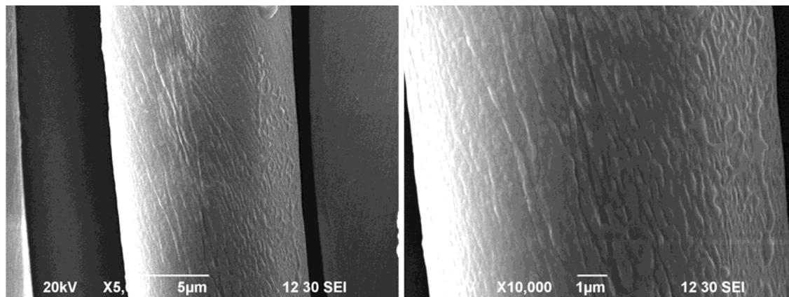
**Fig. 4.** SEM micrographs of original cotton fibres captured at magnification of 5,000x and 10,000x
