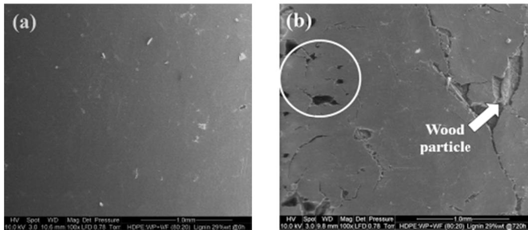
**Fig. 7.** SEM micrographs of surfaces of WPE composites of lignin content of 29 %wt. before and after UV weathering at 100x magnification: (a) Before UV weathering; (b) After 720 h UV weathering time
