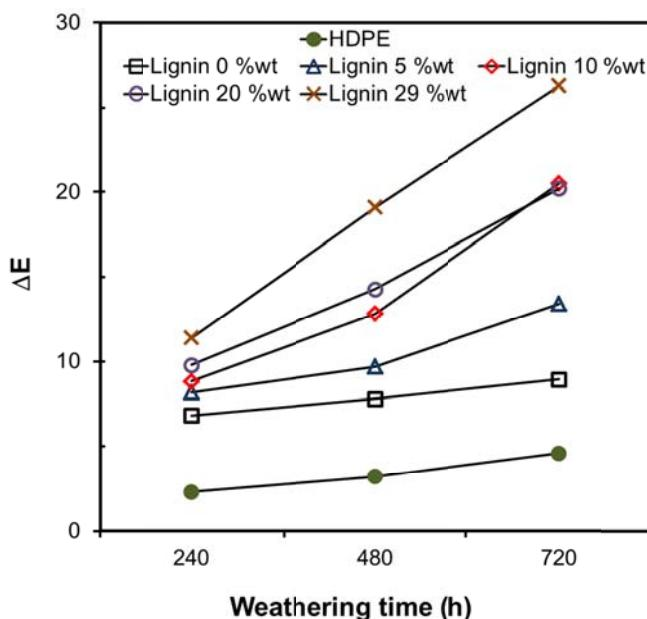
**Fig. 2.** Discoloration level of HDPE and WPE composites of various lignin contents as a function of UV weathering times
