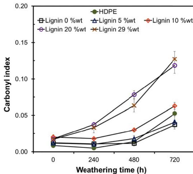
**Fig. 4.** Effect of lignin content on carbonyl index in HDPE and WPE composites
