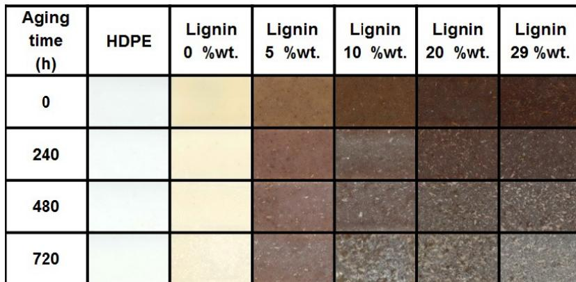
**Fig. 3.** Digital photos of HDPE and WPE composite specimens at different UV weathering times
