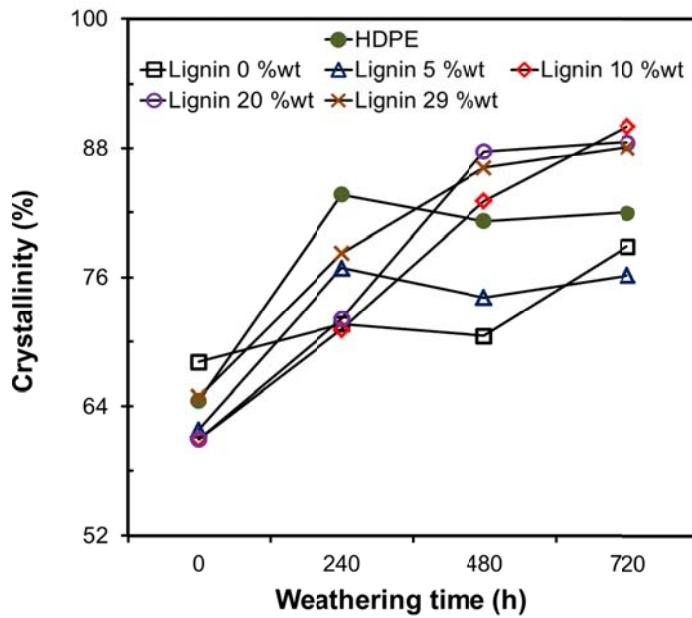
**Fig. 9.** Percentage crystallinity of HDPE in HDPE and WPE composites as a function of UV weathering times by DSC analysis
