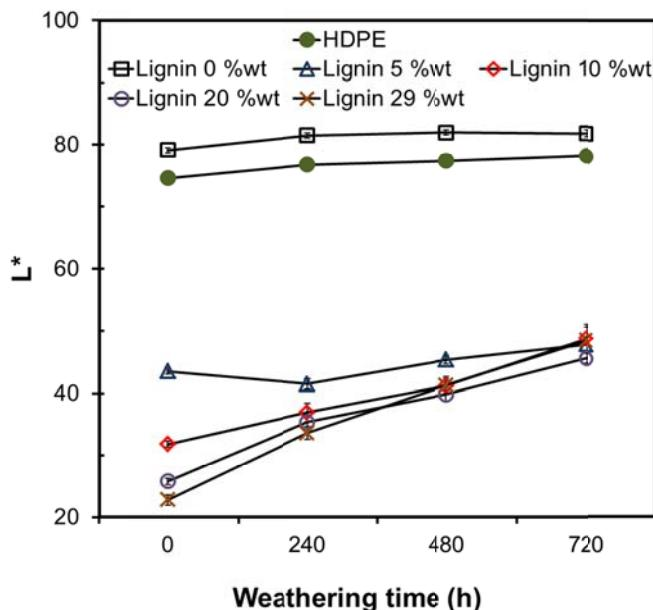
**Fig. 1.** Lightness of HDPE and WPE composites of various lignin contents as a function of UV weathering times
