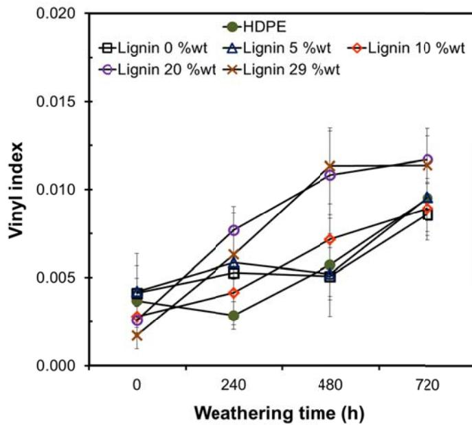
**Fig. 5.** Effect of lignin content on vinyl index in HDPE and WPE composites
