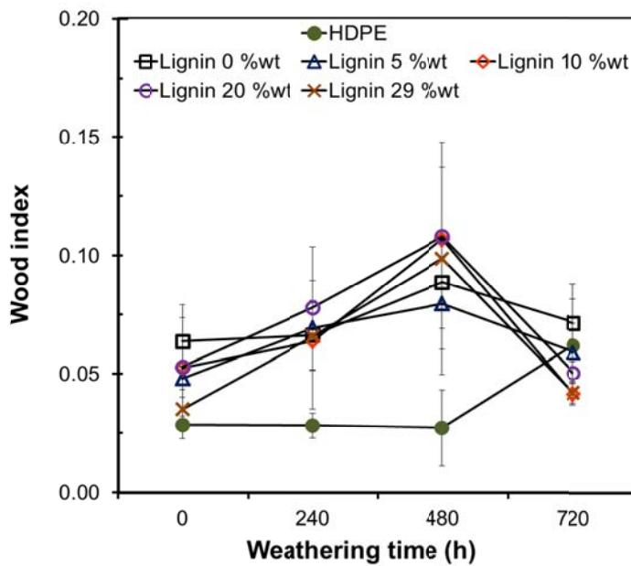
**Fig. 6.** Wood index of surface of WPE composites at different UV weathering times
