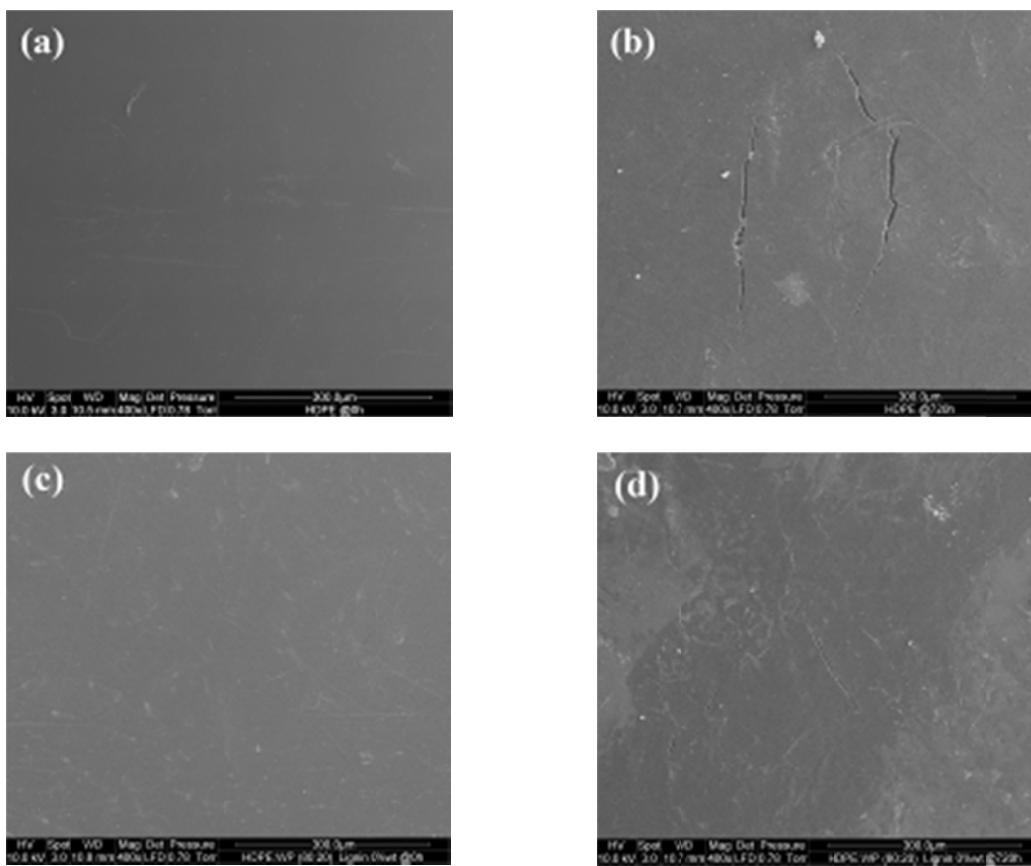
**Fig. 8 (a-d).** SEM micrographs of surfaces of neat HDPE and WPE composites before and after UV weathering at 400x magnification: (a), (c), (e), and (g) before UV weathering of neat HDPE and WPE composites of lignin content of 0, 5, and 29 %wt., respectively; (b), (d), (f), and (h) after 720h UV weathering time of neat HDPE and WPE composites of lignin content of 0, 5, and 29 %wt., respectively
