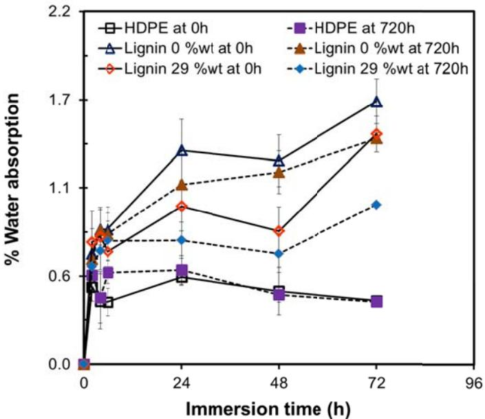
**Fig. 11.** Water absorption of HDPE and WPE composites before and after 720 h UV weathering time
