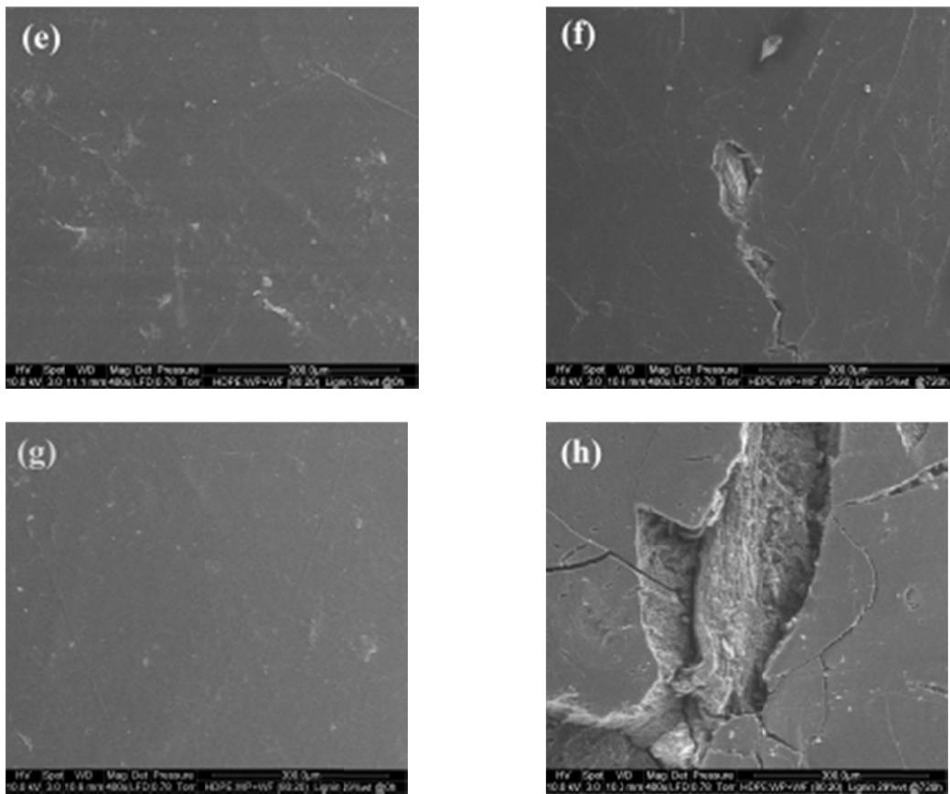
**Fig. 8 (e-h).** SEM micrographs of surfaces of neat HDPE and WPE composites before and after UV weathering at 400x magnification: (a), (c), (e), and (g) before UV weathering of neat HDPE and WPE composites of lignin content of 0, 5, and 29 %wt., respectively; (b), (d), (f), and (h) after 720h UV weathering of neat HDPE and WPE composites of lignin content of 0, 5, and 29 %wt.
