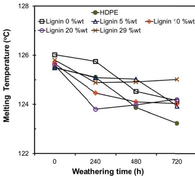
**Fig. 10.** The onset melting temperatures of HDPE and WPE composites as a function of UV weathering times
