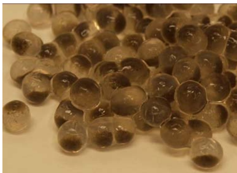
Fig. 1. Capsules made of natural membrane, containing digesting bacteria
