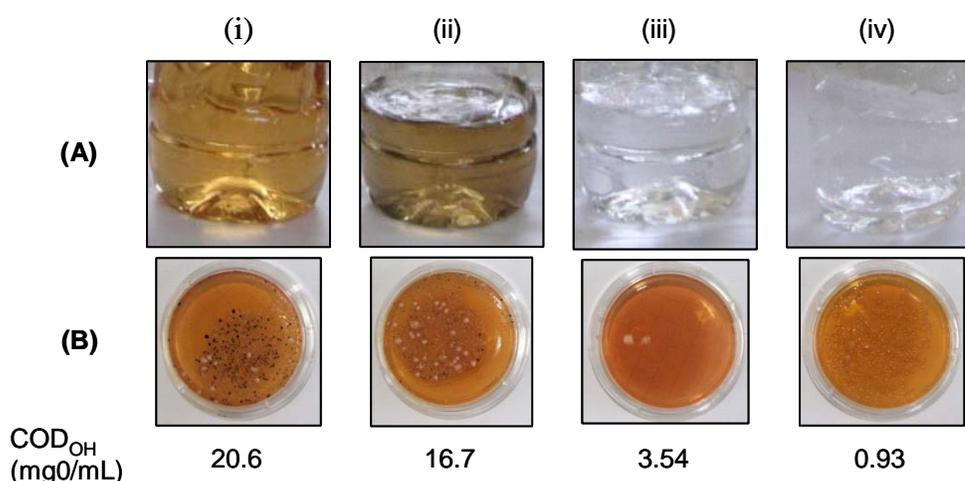
**Figure 5.** Decoloration (A) and bacterial colonization of the creek water in University of Palangka Raya purified by type B apparatus. See detail of this apparatus in Figure 2. (i), after purification with keranggas; (ii), with keranggas followed by charcoal; (iii), with charcoal followed by AC with 870 mg/g of iodine adsorption; (iv), with AC followed by keranggas. The initial  $COD_{OH}$  of this creek water was 20.0 mgO/mL.
