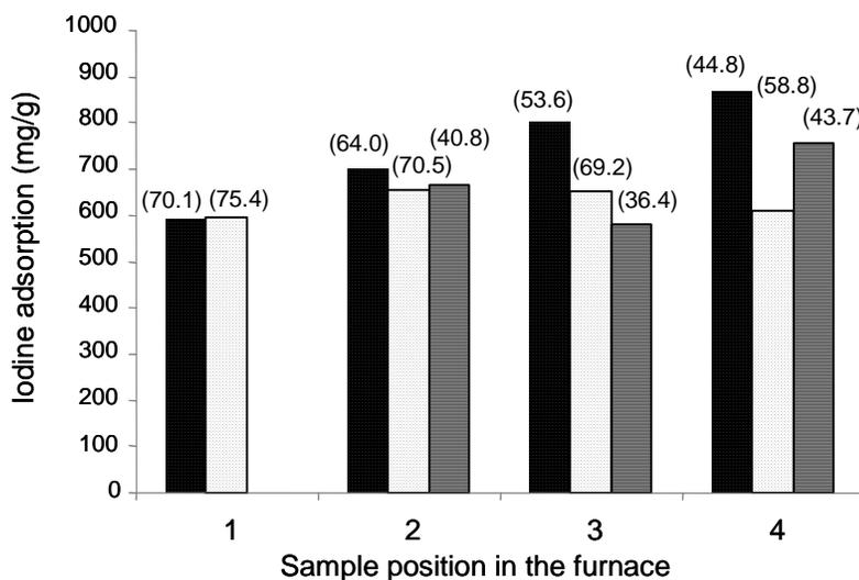
**Figure 3.** Iodine adsorption and yield of AC from wood charcoal.
