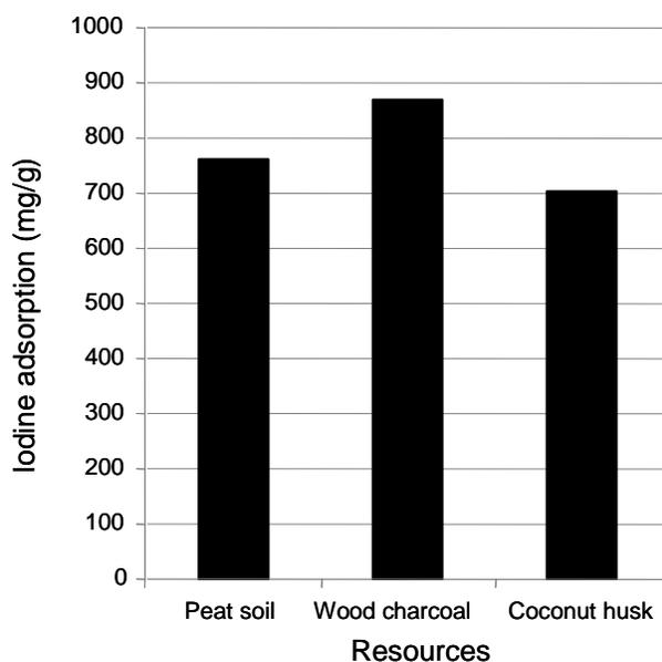
**Figure 4.** Iodine adsorption of AC from different raw materials.
