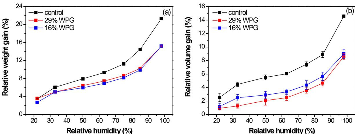
**Fig. 2.** Relative gains of weight (a) and volume (b) of the wood- $\text{TiO}_2$  composites with different WPGs (control, black line; 16% WPG, blue line; 29% WPG, red line) during storage in ambient atmosphere with varied relative humidity (RH). Values are given as mean of 10 replicates with the standard deviation as error bars. For part (a) no error bars are shown, since the intervals were small relative to the size of the plotted points.
