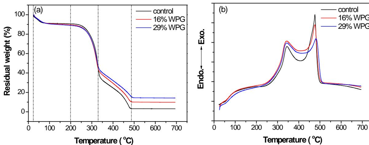
**Fig. 3.** Thermal behavior (a, TG curve; b, DTA curve) of wood-TiO<sub>2</sub> composites with different WPGs (control, black line; 16% WPG, red line; 29% WPG, blue line)
