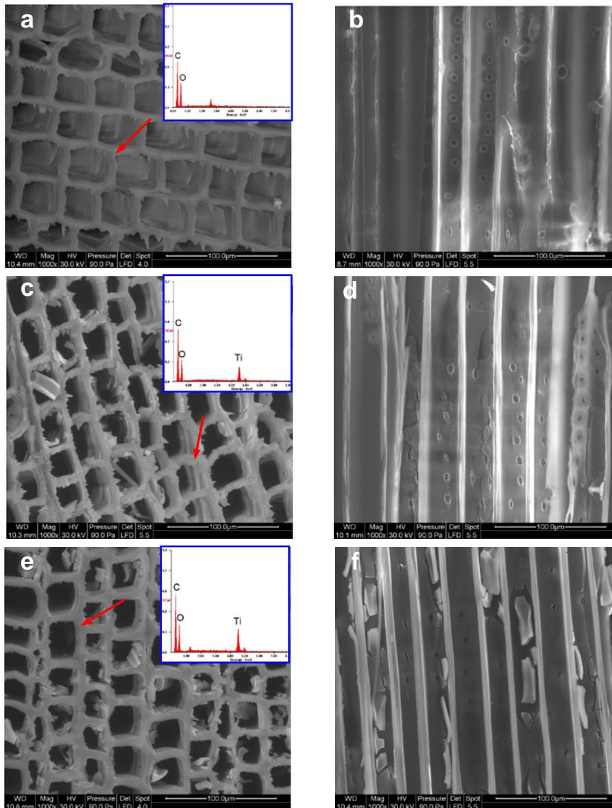
**Fig. 1.** ESEM images of wood- $TiO_2$  composites with weight percentage gain (WPG) of 16% (c, d) and 29% (e, f) in comparison with the untreated control (a, b). Cross section (a, c, e), radial section (b, d, f). The inserted pictures are the corresponding EDAX spectra of cell walls.
