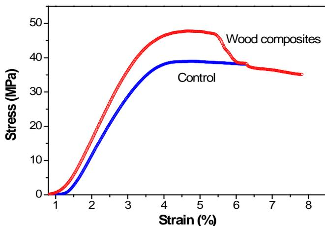
**Fig. 4.** Typical stress-strain curves of wood-TiO<sub>2</sub> composites (red line, upper) and untreated control (blue line, lower) under compression in the longitudinal direction
