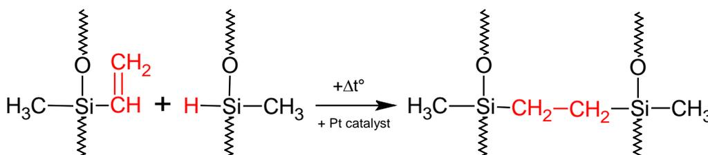
Fig. 3. Silicone thermal addition cure chemistry
