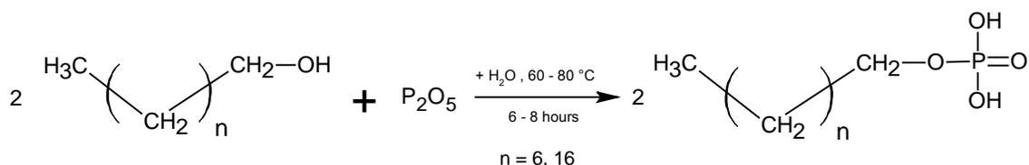
**Fig. 4.** Phosphate esters synthesis reaction
