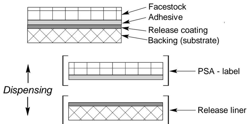
**Fig. 1.** Structure of a self-adhesive label laminate
