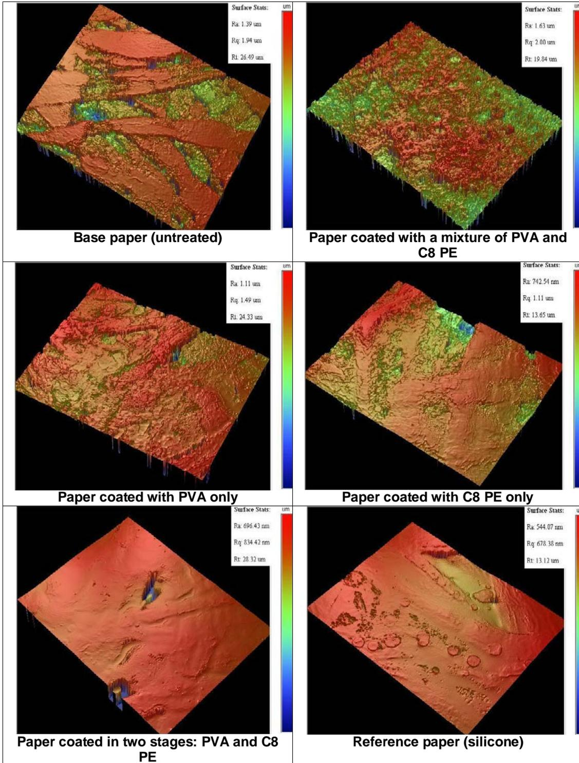
**Fig. 6.** Surface topography of paper treated with different coating formulations
