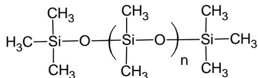
**Fig. 2.** Chemical structure of polydimethylsiloxane (PDMS)
