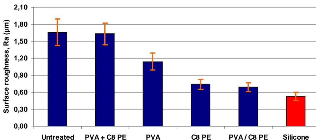
Fig. 7. Changes in paper surface roughness as result of the coating process
