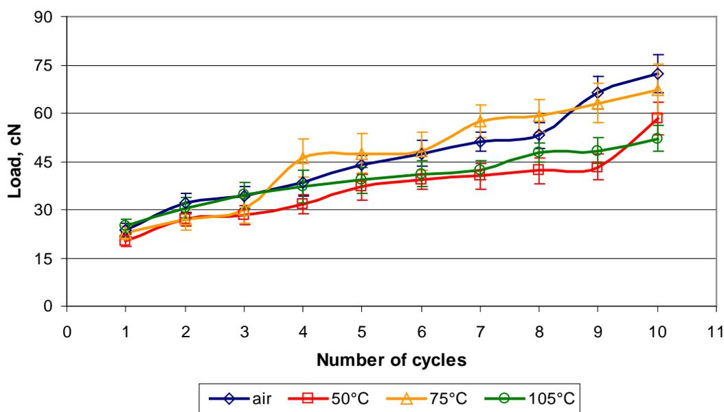
**Fig. 5.** Influence of thermal treatments and number of peel test cycles on the peel force value
