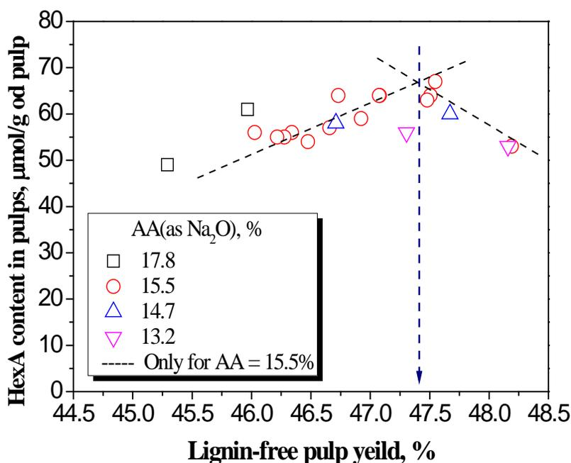
Fig. 2. The change of HexA content with lignin-free pulp yield
