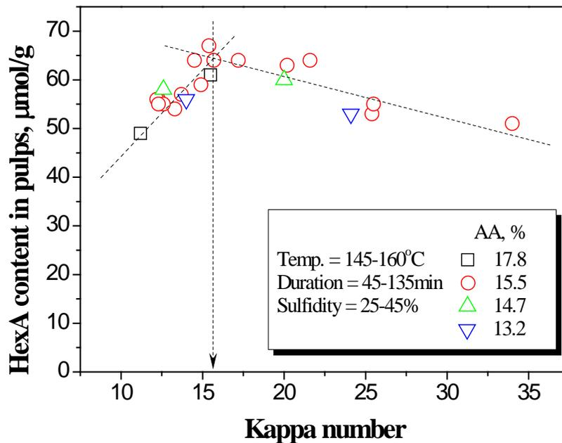
Fig. 4. The formation and dissolving of HexA with kappa number change of pulps
