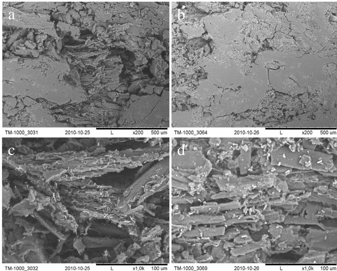
**Fig. 5.** Scanning electron microscope micrographs at two different magnifications of the surface of WPC specimens with an unmodified (a, c) and acetylated (b, d) wood component, artificially aged by weathering, water soaking, and followed by a brown-rot fungus exposure (U4, A4)
