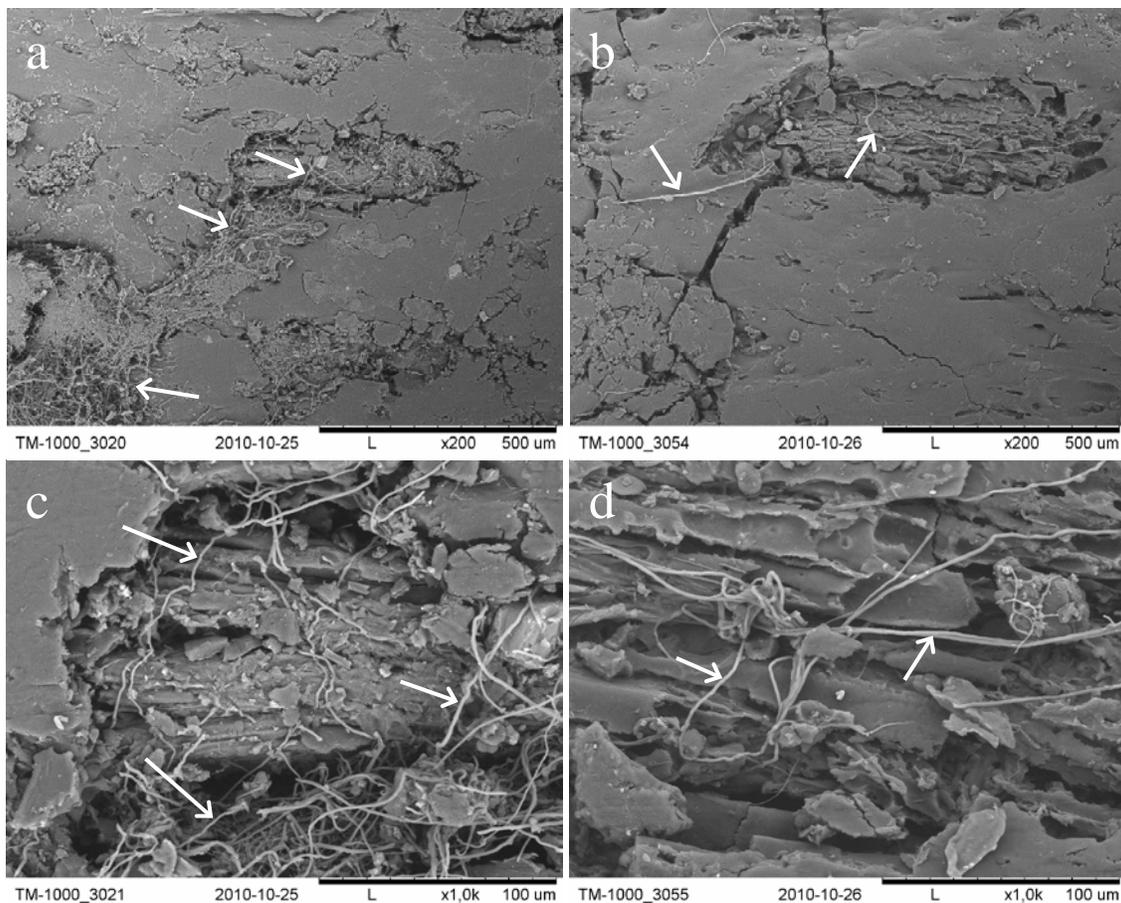
**Figure 4.** Scanning electron microscope micrographs at two different magnifications of the surface of WPC specimens with an unmodified (a, c) and acetylated (b, d) wood component, artificially aged by weathering, water soaking, and followed by a white-rot fungus exposure (U3, A3). White arrows indicate fungal hyphae.
