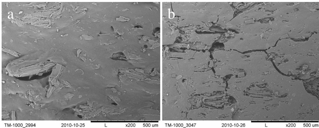
**Fig. 3.** Scanning electron microscope micrographs of the surface of WPC specimens with an unmodified wood component, artificially aged by a) water soaking (U1) and b) weathering followed by water soaking (U2)
