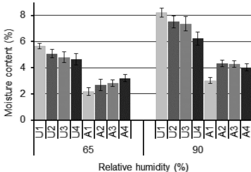
Fig. 1. Equilibrium moisture content of the WPC samples in either 65% or 90% relative humidity
