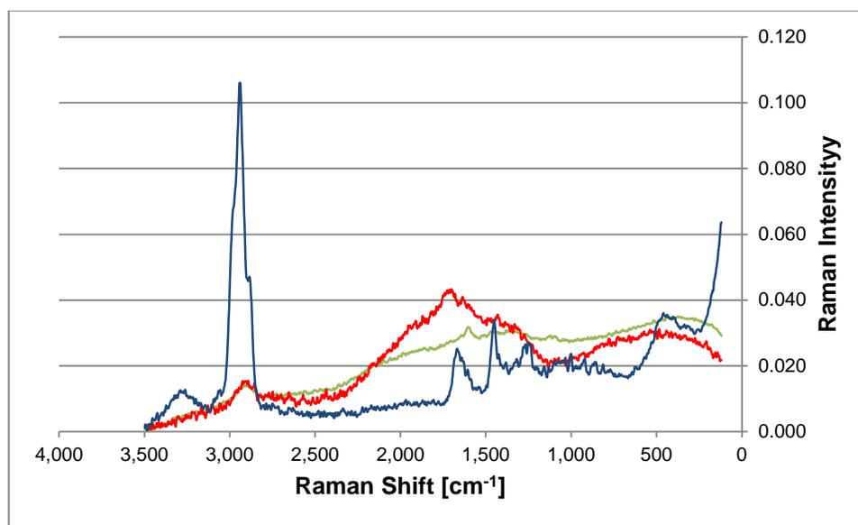
Fig. 1. Averaged Raman spectra of lignin (red), wood (green), and leather (blue)
