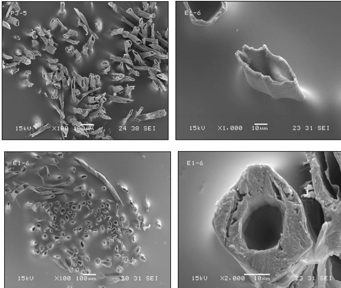
Fig. 13. Cross-section of EW (upper) and LW (lower) R28 fraction fibers
