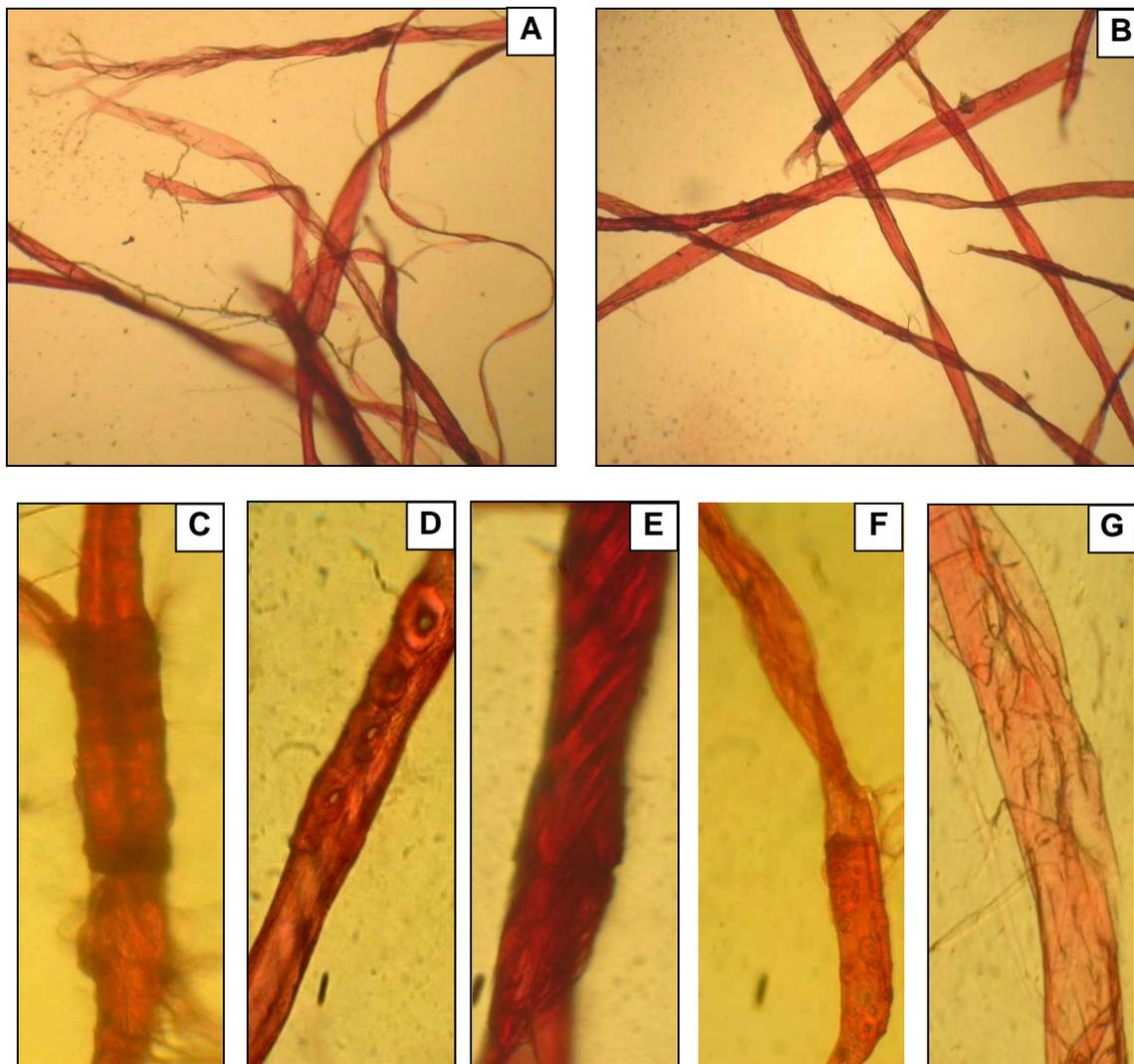
**Fig. 6.** Micrographs showing the surface characteristics of fibres of LW and EW in R48 fractions (A): LW R48 fibre (x40); (B): EW R48 fibres (x40); (C) "Sleeve rolling" effect on LW fibre (x160); (D) Partly peeled LW fibre (x160); (E): Fibrillated S2 layer in LW fibre, spiral cracks in fibre wall (x160); (F): A twisted and fibrillated EW fibre (x160); (G): Wall-fractured and split EW fibre (x160).
