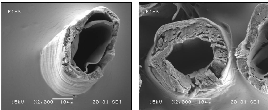
**Fig.12.** Internal fibrillation of EW (left) and LW (right) fibers
