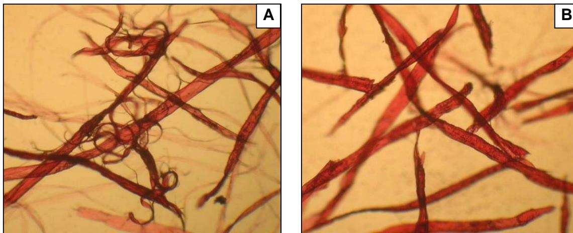
**Fig. 7.** Micrographs showing the nature of the fibres of R100 fraction of LW and EW: (A): LW R100 fraction showing fibrillated fibre ends and large bands of fibrils (x40); (B): EW R100 fraction showing broken fibre with little fibrils (x40).
