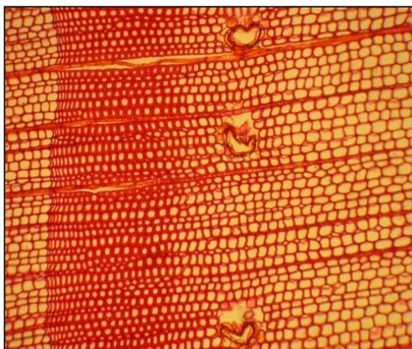
Fig. 1. Cross-section morphology of EW (left) and LW (right) of Jack pine (x200)
