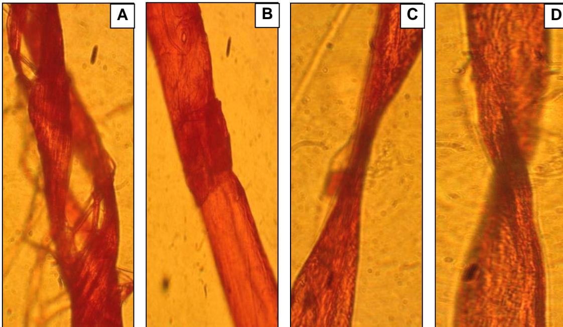
Fig. 3 (A-D). Micrographs showing the surface characteristics of LW fibres in R14 fraction (x400)
