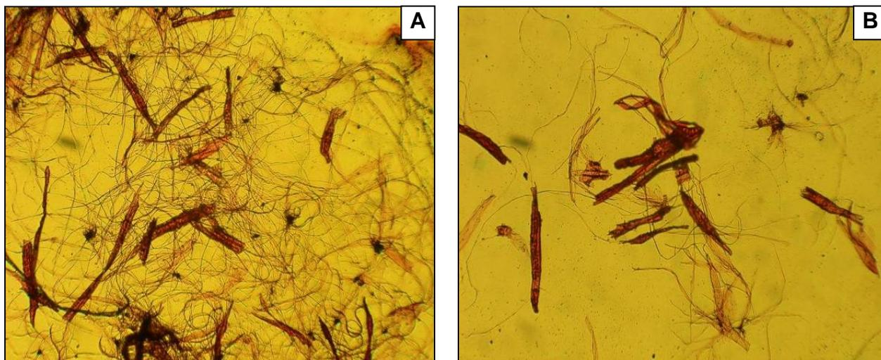
**Fig. 8.** Micrographs showing the nature fibrous elements of LW and EW fibres in R200 fractions (A): LW R200 fraction showing chunky developed fibre with bands of fibrils (x40); (B): EW R200 fraction showing under-developed fibres and little fibrils (x40).
