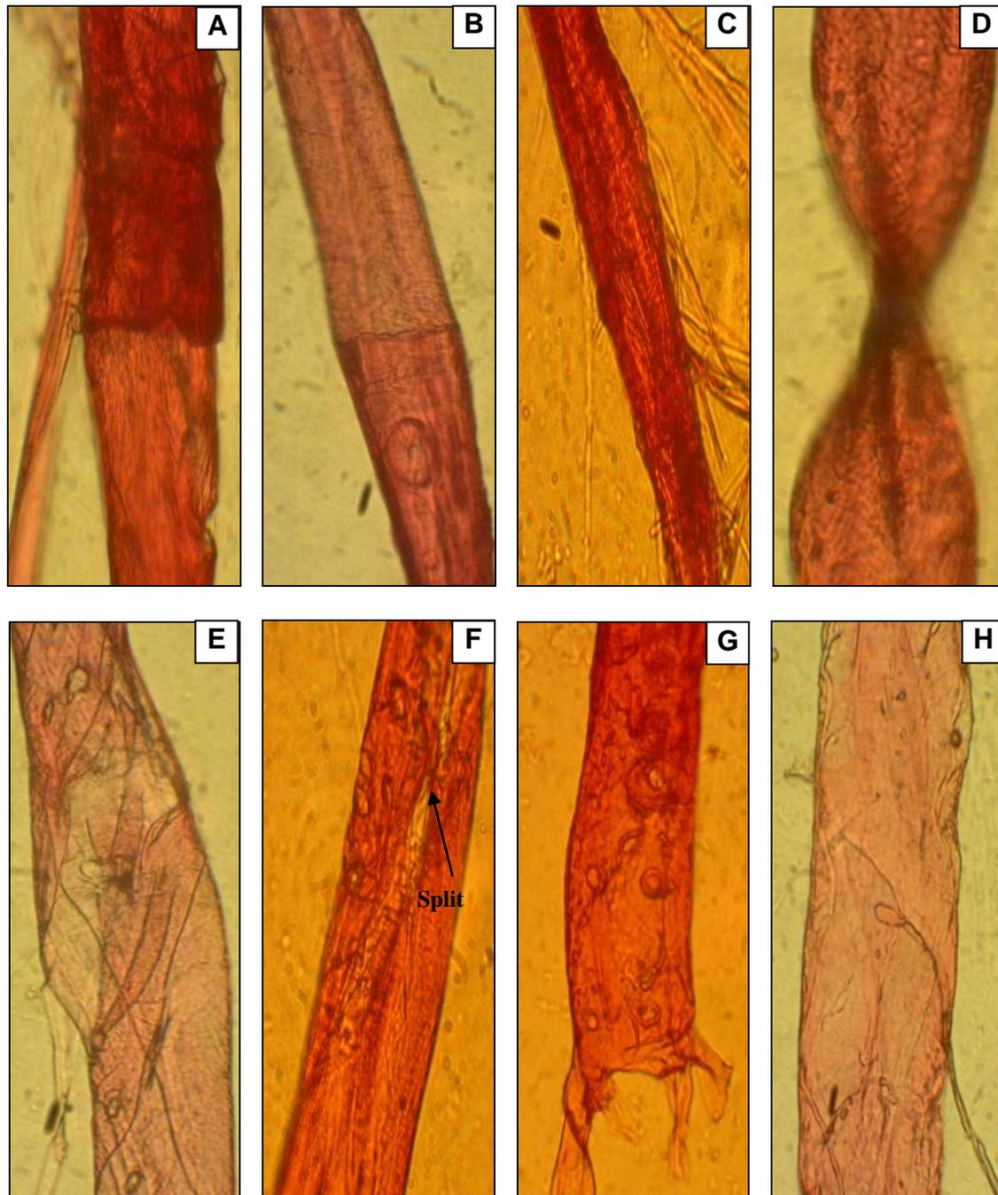
**Fig. 5.** Micrographs demonstrating the refining effect on R28 fraction of LW and EW fibres (x400)
