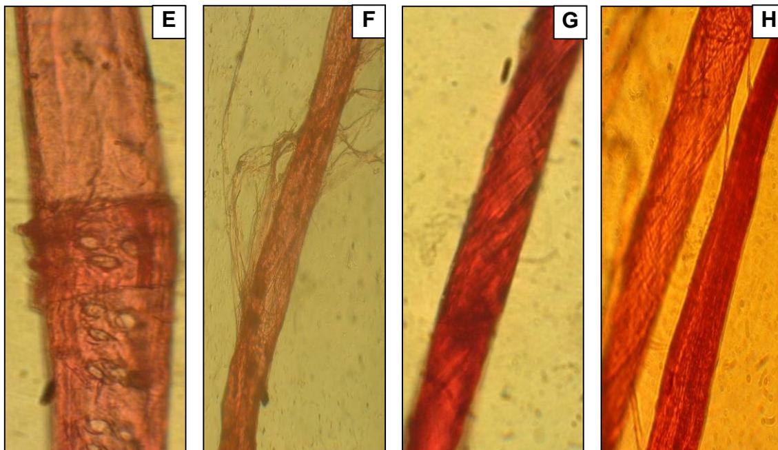
**Fig. 3 (E-H).** Micrographs showing the surface characteristics of LW fibres in R14 fraction (x400)
