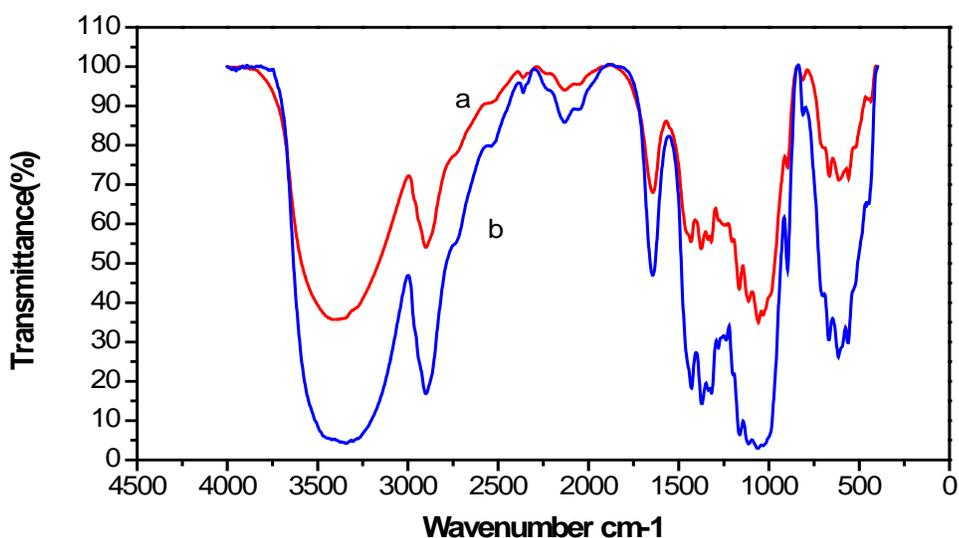
Fig. 4. FTIR spectra of bamboo nanocrystalline cellulose (a), and bamboo pulp with NaOH pretreatment (b)
