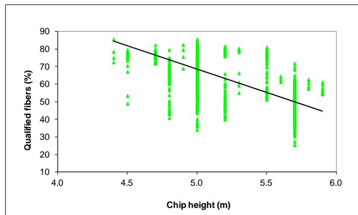
Fig. 7. The relationship between qualified fibers and chip height
