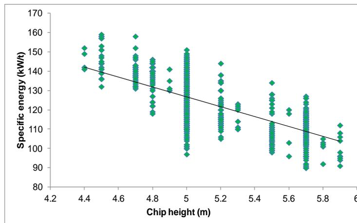
**Fig. 4.** The relationship between the specific energy consumption and chip height
