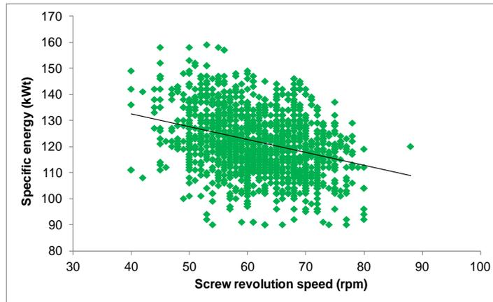
**Fig. 5.** The relationship between the specific energy consumption and screw revolution speed
