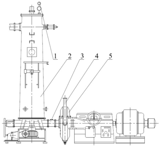
**Fig. 1.** The major components of the refiner: 1. Pressure meter of the pre-heater; 2. Pre-heater; 3. Feeding pipe; 4. Discharging pipe; and 5. Refiner
