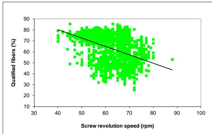
**Fig. 8.** The relationship between qualified fibers and feeding screw resolution
