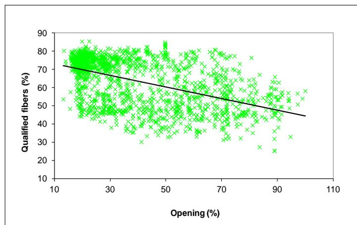
Fig. 6. The relationship between qualified fibers and valve opening
