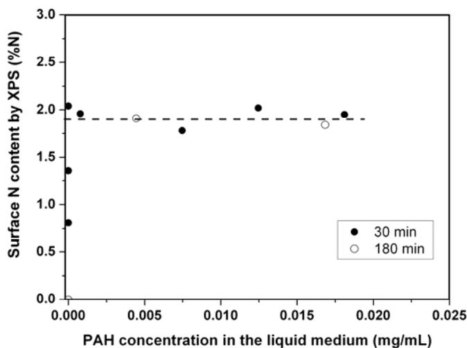
**Fig. 2.** Surface nitrogen content determined by XPS as a function of PAH equilibrium concentration where PAH adsorption took place, at pH 7.5, NaCl 0.01N for 30 and 180 min
