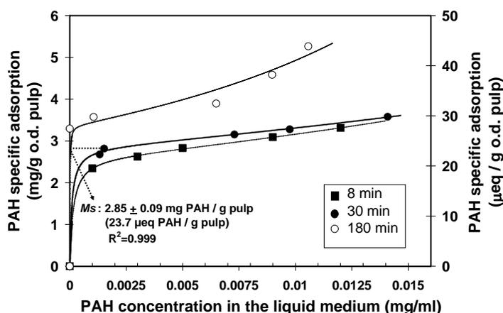
**Fig. 1.** PAH specific adsorption as a function of PAH equilibrium concentration at different times, pH 7.5 and NaCl 0.01N. Equation (1) was fitted to data points to obtain the values of the parameters. The amount of PAH is expressed in mg PAH/g pulp, and in  $\mu\text{eq}$  PAH /g pulp, considering a charge density of 8.30 meq/g PAH.
