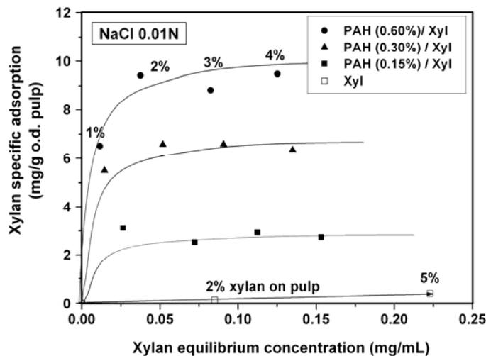
**Fig. 4.** Xylan specific adsorption on untreated and on previously PAH treated pulps as a function of the xylan equilibrium concentration at pH 7.5 and NaCl 0.01N. Dosages of the commercial xylan are indicated in the plot (% xylan on pulp). In this case, the dosage 0.3 % PAH on pulp corresponds to saturation of fiber surface charges when the ionic strength corresponds to 0.01N NaCl.
