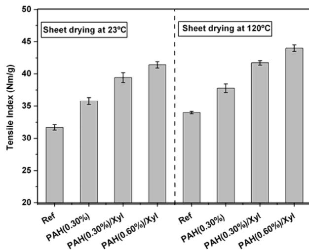
**Fig. 8.** Tensile strength as a function of the different treatments at 23°C or 120°C, pH 7.5 and 0.01N NaCl. The error bars correspond to the standard deviations of the means from ten replications of the trial.
