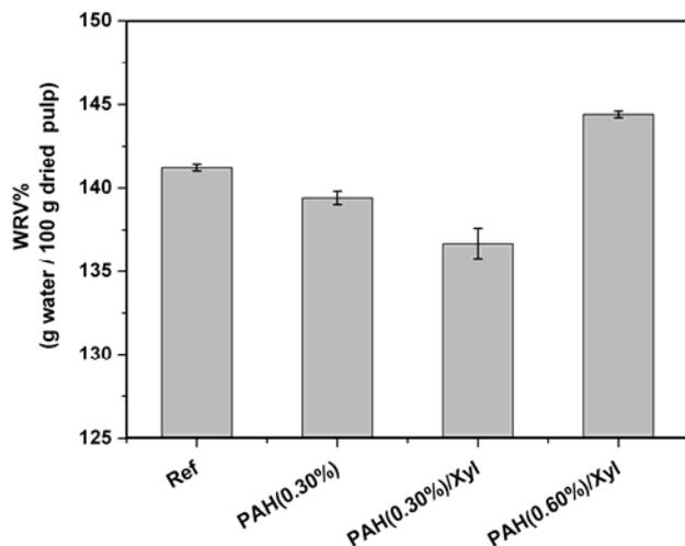
**Fig. 7.** Effects of PAH and PAH/Xylan treatments on water retention values at pH 7.5 and NaCl 0.01N. The error bars correspond to the standard deviations of the means from three replications of the trial.
