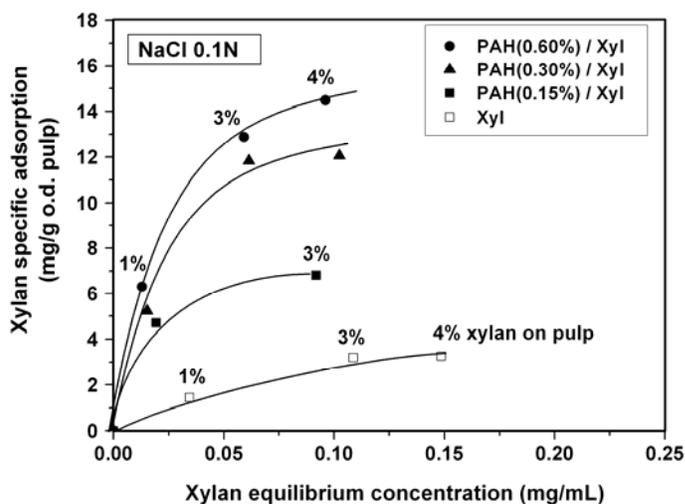
**Fig. 5.** Xylan specific adsorption on untreated and on previously PAH treated pulps as a function of the xylan equilibrium concentration at pH 7.5 and NaCl 0.1N. Dosages of the commercial xylan are indicated in the plot (% xylan on pulp).
