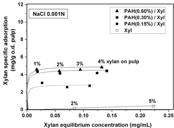
**Fig. 3.** Xylan specific adsorption on untreated and on previously PAH treated pulps as a function of the xylan equilibrium concentration at pH 7.5 and NaCl 0.001N. Dosages of the commercial xylan used are indicated in the plot (% xylan on pulp).
